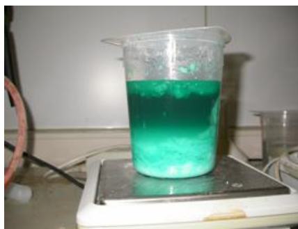
Figure 2.8 Floating Ice and settled nickel sulfate inside the crystallizer.
