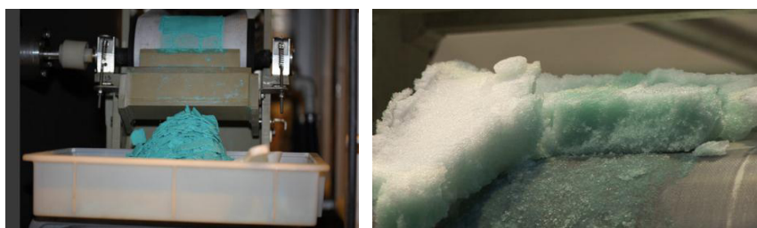
Figure 2.10 Nickel sulfate (left) and ice (right) on the belt filter.
