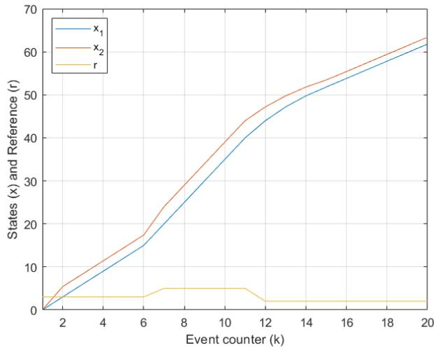
**Figure 5-3:** Closed-loop control of a production system using input strategy 1
