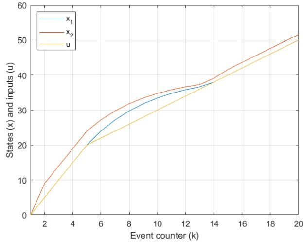
**Figure 4-5:** Open-loop control of a production system using input strategy 1
