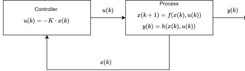
**Figure 5-1:** Schematic overview of a closed-loop control system
