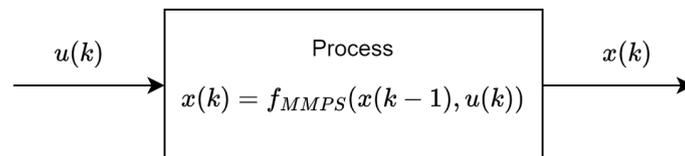
**Figure 4-3:** Schematic overview of an open-loop MMPS system
