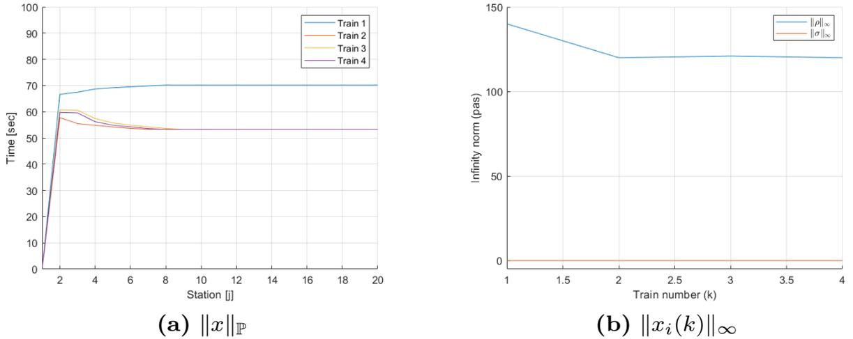
**Figure 8-7:** Hilbert's projective norm and infinity norm for the simulation of the autonomous URS from unstable initial conditions
