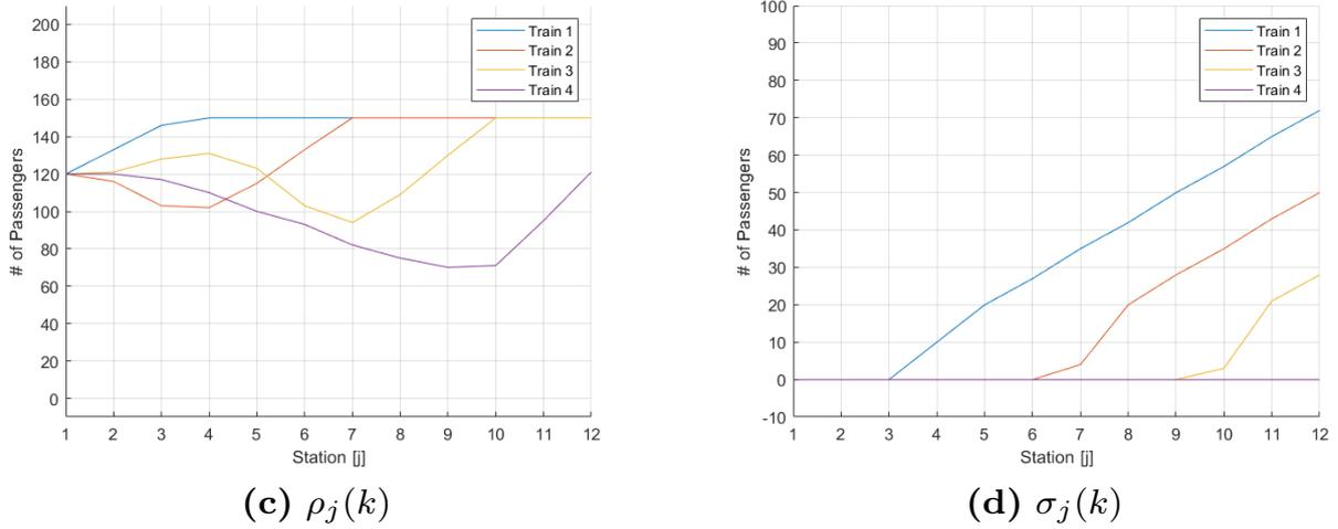
**Figure 8-3:** States and objective for the autonomous URS simulated from unstable initial conditions
