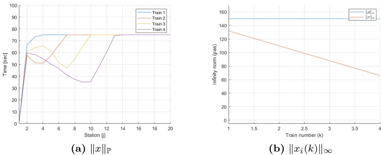
**Figure 8-4:** Hilbert’s projective norm and infinity norm for the simulation of the autonomous URS from unstable initial conditions
