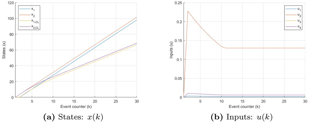
**Figure 6-1:** Simulation autonomous and closed-loop production system from  $x_0 = [0, 0]^T$
