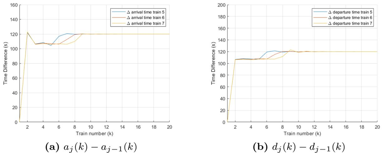
**Figure 8-9:** Difference in arrival and departure times between stations, closed-loop system
