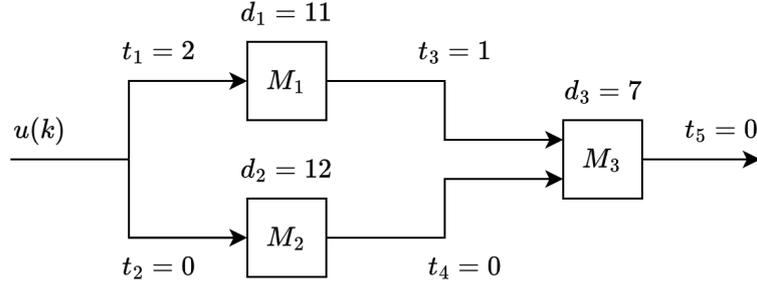
**Figure 7-1:** Simple Manufacturing System
