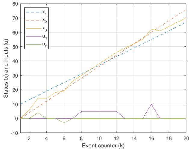
**Figure 4-8:** Open-loop control of a production system using input strategy 3
