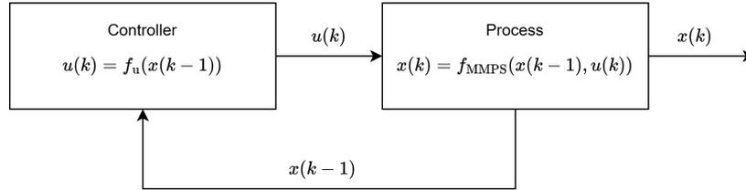
**Figure 5-2:** Schematic overview of a closed-loop explicit MMPS system
