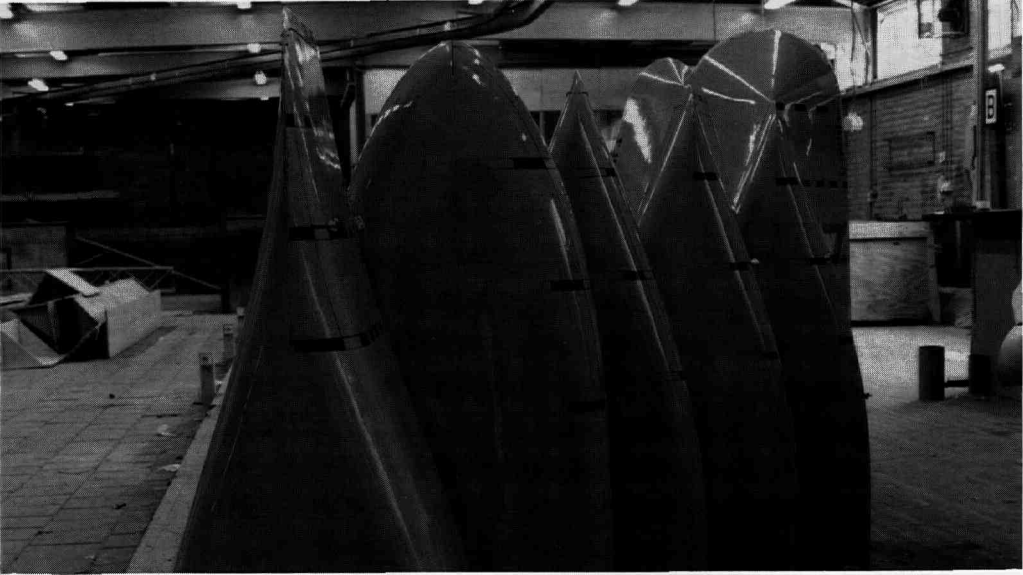
Photo 7.7.2-1: Forebody sections of models.
