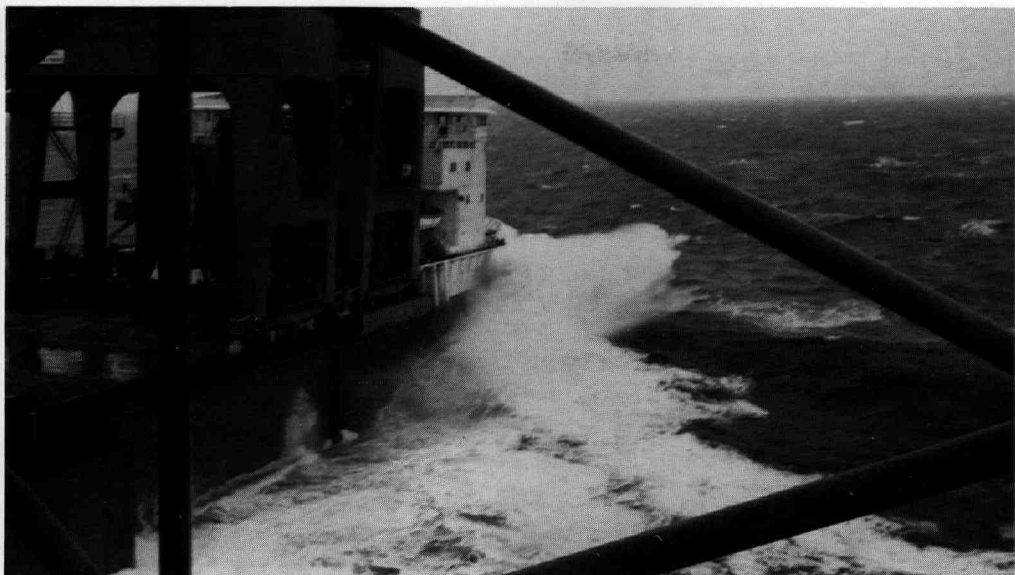
A heavy-load ship in a moderate seaway; view taken from jack-up drilling rig deck cargo, looking forward at the bow, [Courtesy Dock-Express Shipping B.V., Rotterdam].
