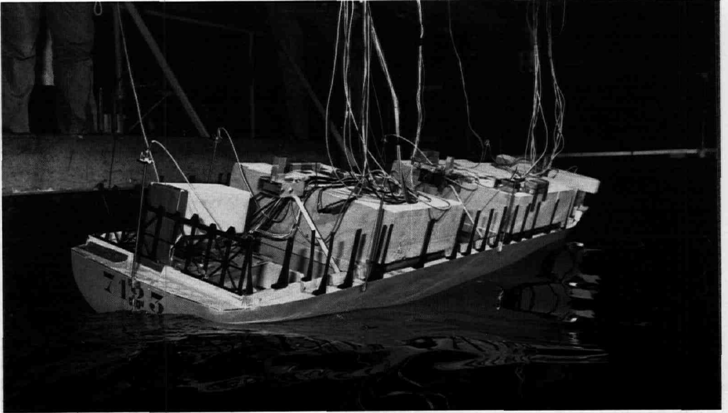
Photo 1-2: Oscillatory ship motions and orbital wave motion will produce an oscillatory inflow into the propeller [open containership model in waves, courtesy Verolme Shipyards Heusden B.V.]
