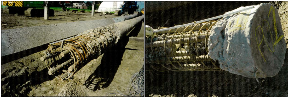
Figure 6.1: Photos of the piles after tension tests at the Gaag viaduct in Schipluiden. Noticeable deterioration of concrete towards the pile tip was observed (Geerling and Janse, 1997)
