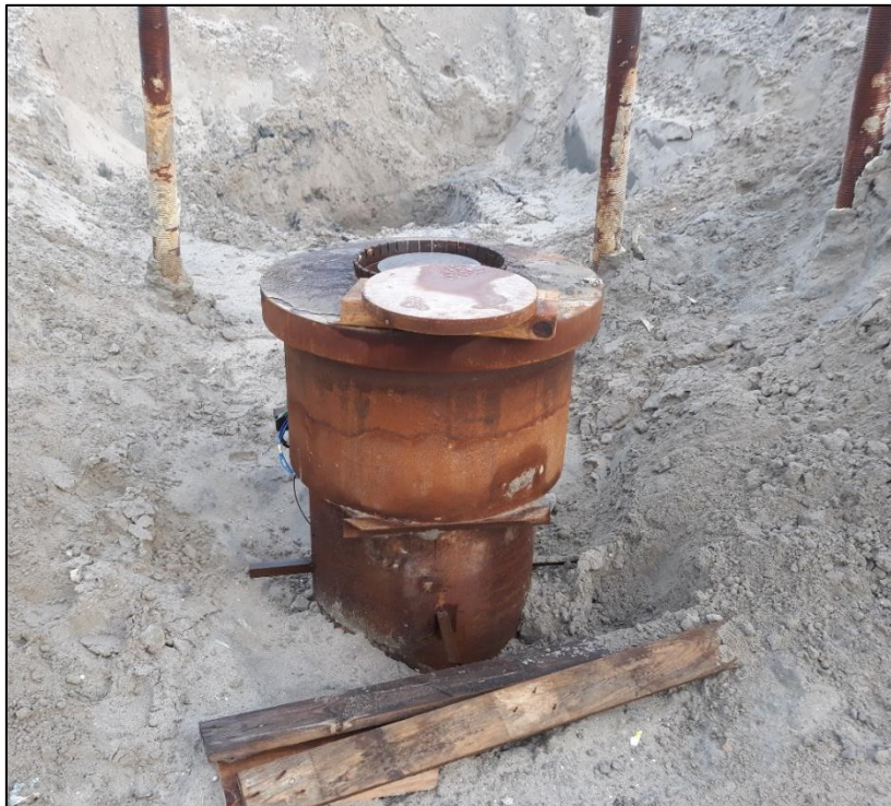
Figure C.6: Vibro pile prepared with pile cap, awaiting installation of the reaction frame
