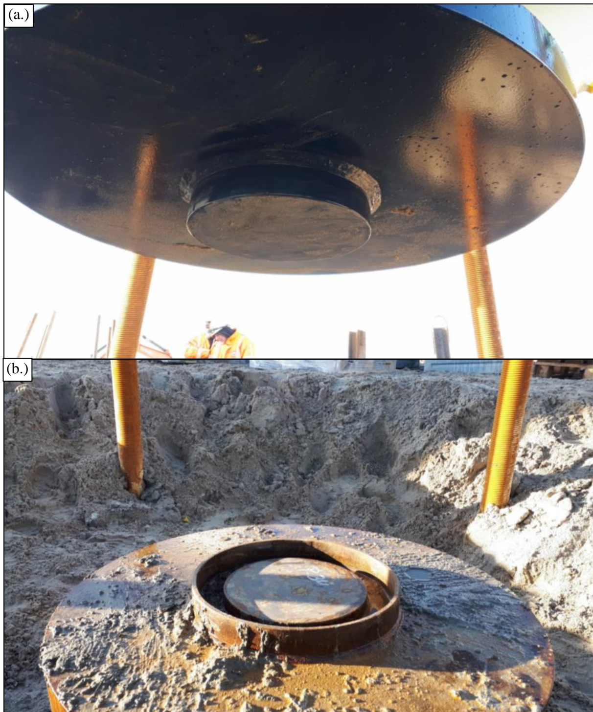
Figure 4.3: Interface between the reaction frame and the pile cap: (a.) underside of the transition piece (b.) top of the pile cap (Photos: Gust Van Lysebetten, WTCB)
