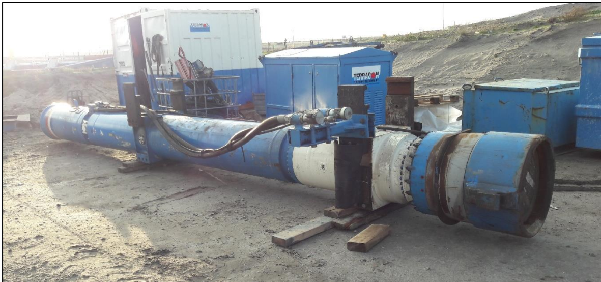
Figure C.2: IHC S-120 hammer used for the installation of the auxiliary tube
