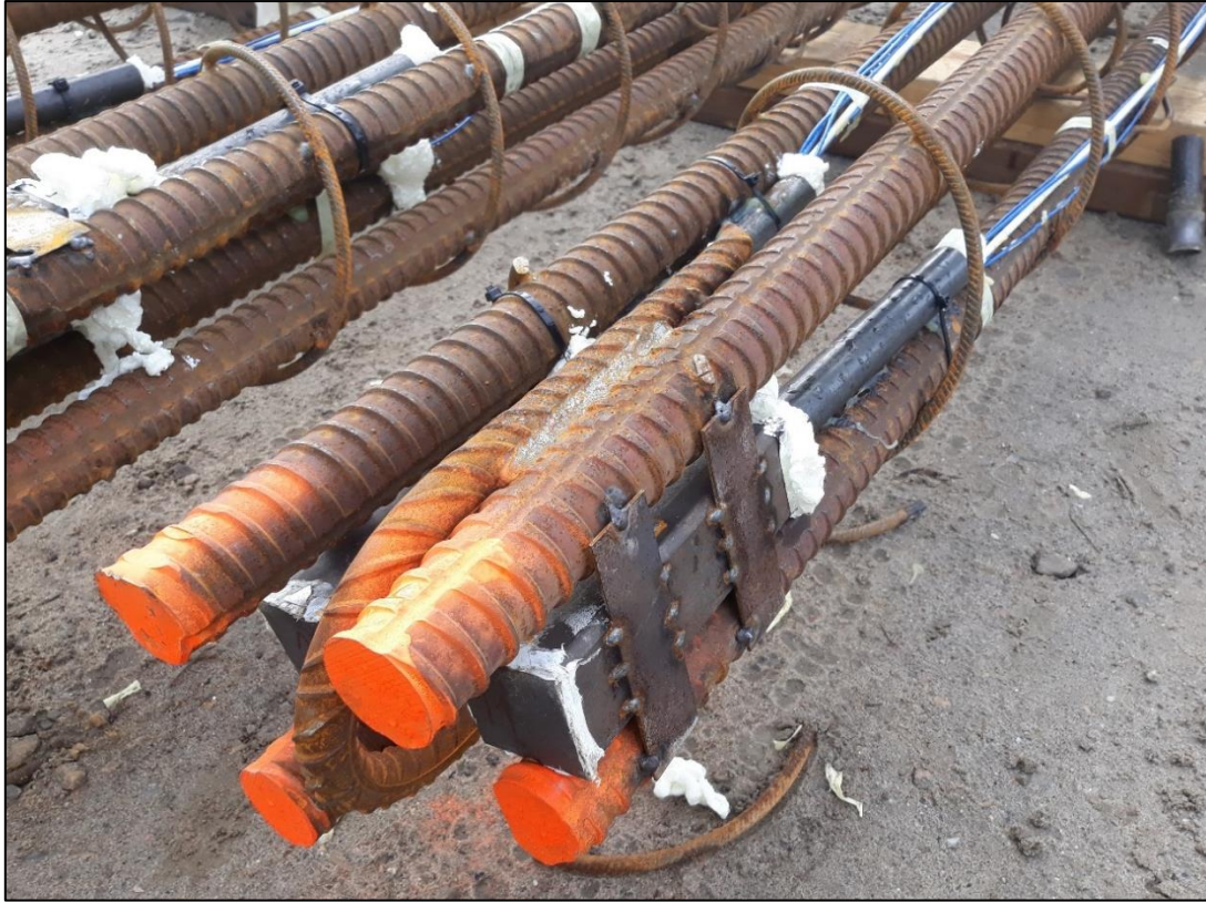
Figure 4.9: The instrumented reinforcement cage in advance of its insertion into the auxiliary tube. Note the two protective metal boxes at the tip of the reinforcement cage.
