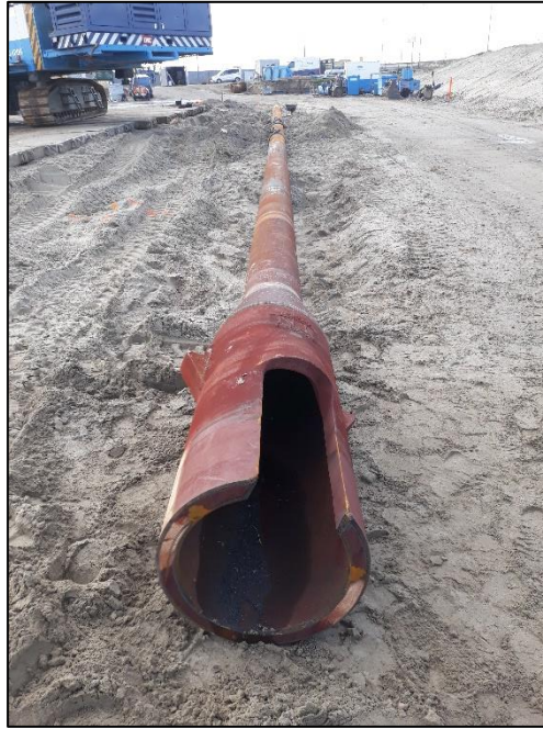
Figure C.1: Head of the steel auxiliary tube lying on the test site prior to pile installation
