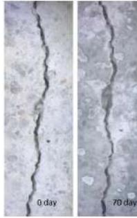
Figure 4.14: Crack width of CEMIII/B based PLA-1 sample.
