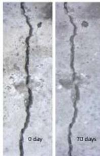
Figure 4.16: Crack width of CEMIII/B based PHA-1 sample.
