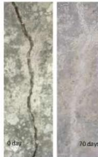
Figure 4.9: Crack width of CEMI based PLA-1 sample.
