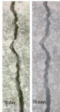
Figure 4.11: Crack width of CEMI based PHA-1 sample.
