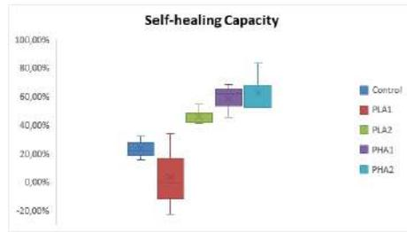
Figure 4.25: Self-healing capacity of CEMIII/B composites.
