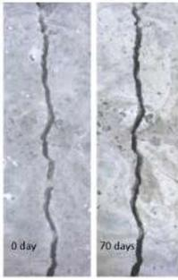
Figure 4.13: Crack width of CEMIII/B based control sample.
