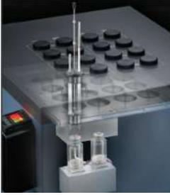
Figure 3.2: A twin type eight channel TAM Air calorimeter with 20ml glass ampoules [4]
