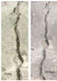
Figure 4.8: Crack width of CEMI based control sample.
