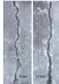
Figure 4.17: Crack width of CEMIII/B based PHA-2 sample.
