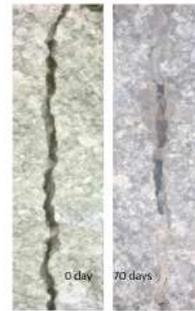
Figure 4.12: Crack width of CEMI based PHA-2 sample.
