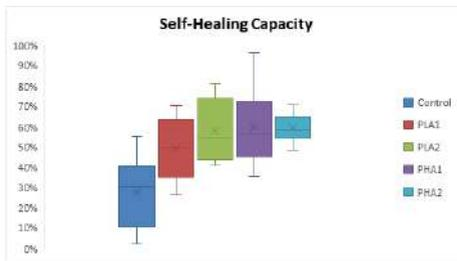
Figure 4.24: Self-healing capacity of CEMI composites.
