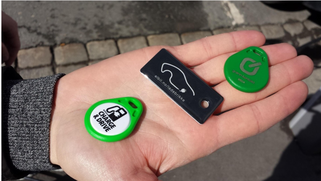
Figure 14: Two charging tags (Fortum and Grønn Kontakt), and a Elbil universal tag.
