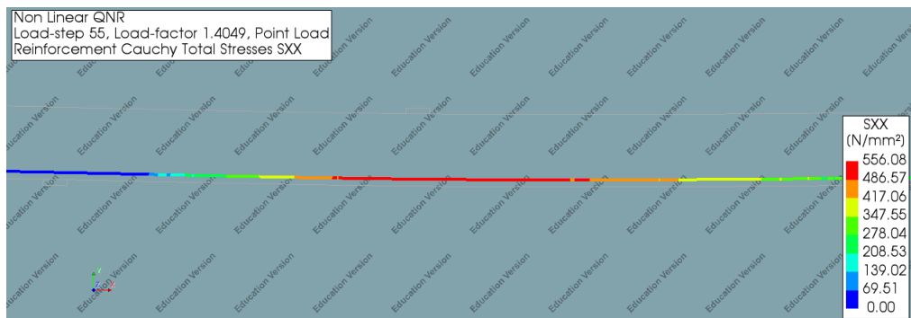
Figure G.6: Reinforcement Stresses at Yielding Step
