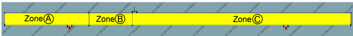
Figure 8.7: Case 2c: Geometry of the NLFEA with localized perturbation of the parameters. CLFM: shear
