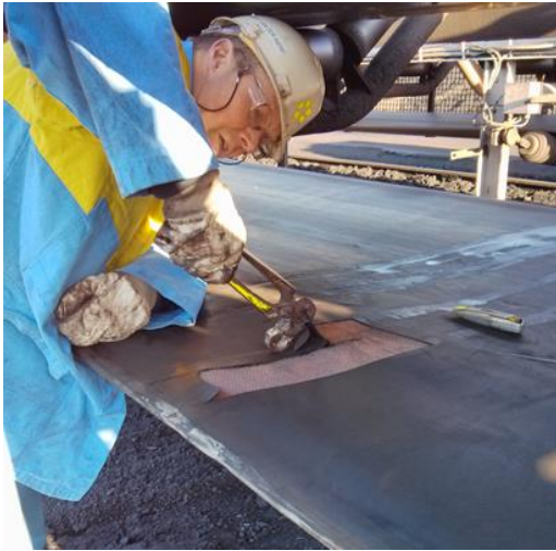
Figure 14: Removing the protective rubber cover
