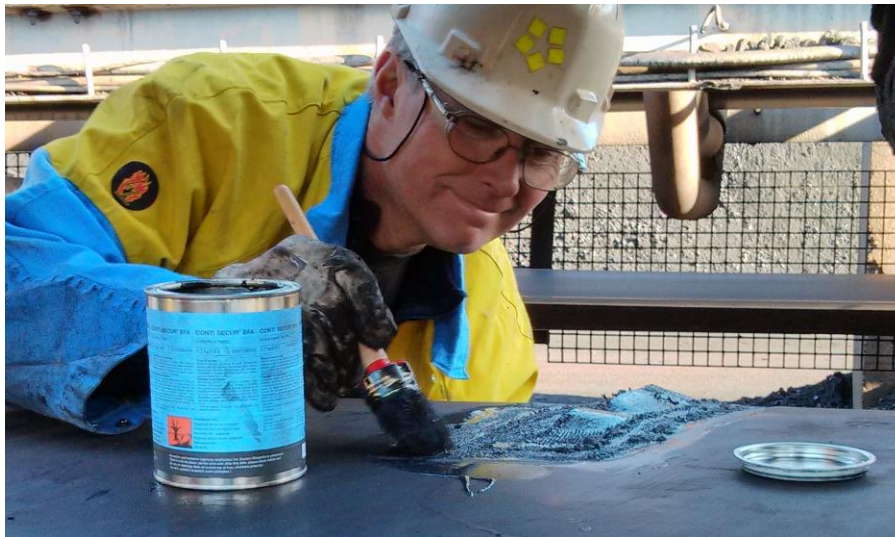
Figure 16: Cementing the fabric before a repair
