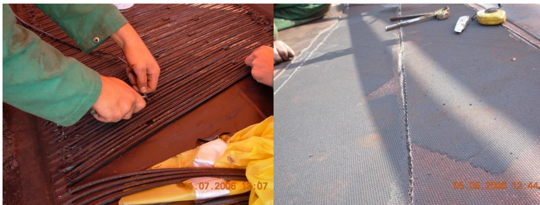
Figure 2: on the left: making of splice in steel cord belt, right: different layers of fabric in fabric belt
