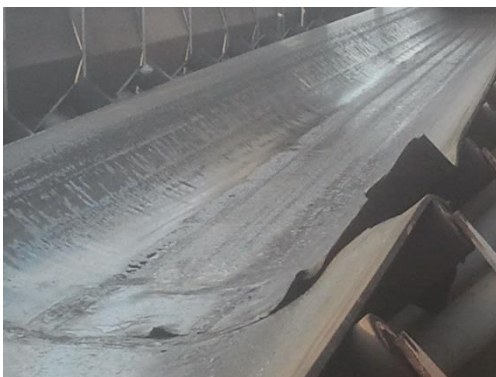
Figure 11: Easily detectible damage to a splice
