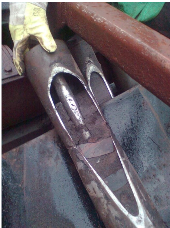
Figure 19: Example of idler rolls that were replaced too late
