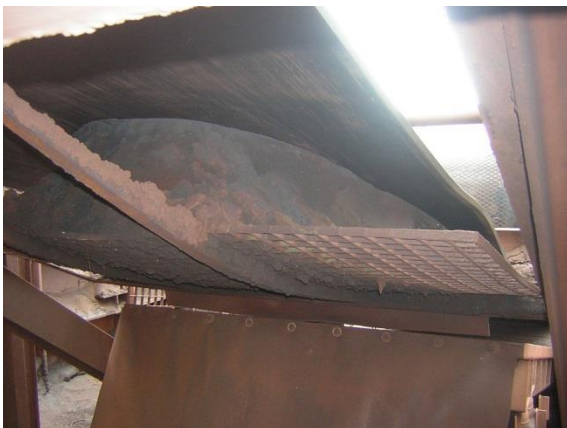
Figure 8: bulk material touching the belt surface
