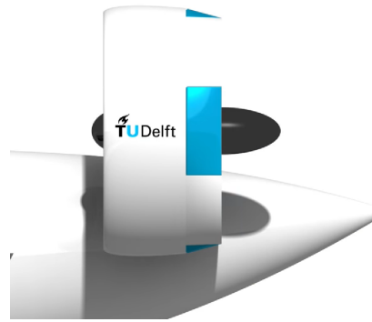
Figure 1.5: DUUC shroud with the control surfaces (shown in blue) incorporated at its surface. Adapted from [57].
