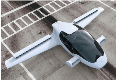
Figure 1.6: Lilium jet distributed propulsion concept [54].
