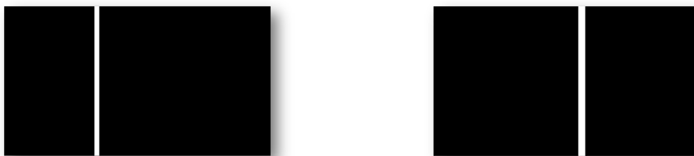
(a) Bitmap image with columns 651 to 685 turned to logical state 1, which corresponds to ON state of the DMD
