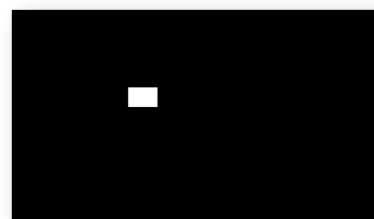
(b) Current output for the bitmap image with 15000 pixels ON was 0.8428 \mu\text{A} . The ON pixels correspond to pixel columns 401 to 500 (100 pixels) and pixel rows 601 to 750 (150 pixels).
