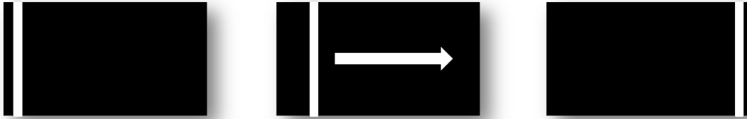
Figure 4.2: Bitmap images corresponding to a monochromatic EQE based modulation scheme. The number of pixel columns turned ON are fixed at 5 and this rectangular white block is scanned along the 1920 pixels as shown above (NOTE - the thickness of the white block in the above image is not 5 pixels, it is exaggerated to 100 pixels for illustration purpose).
