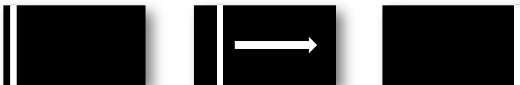
Figure 2.4: Bitmap images of dimensions 1920 pixels (X-direction) \times 1080 pixels (Y-direction) with line scan pattern - the white rectangular block suggests ON micromirrors on the DMD, the rest of the micromirrors are turned OFF.
