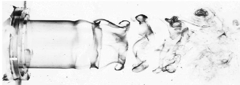
Figure 2.6: Flow visualization of an axi-symmetric turbulent jet.
