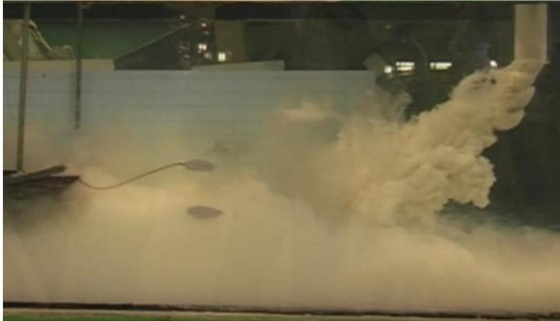
Figure J.2: Plume with halved flume velocity and increased density.
