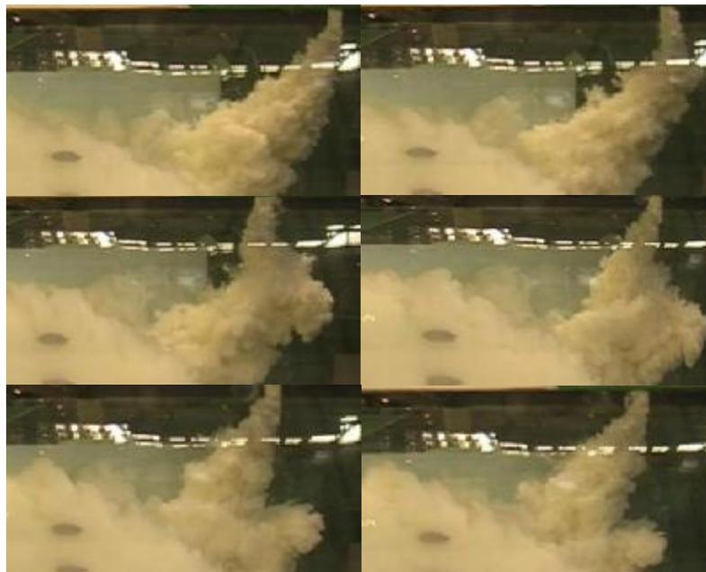
Figure 7.4: Series of subsequent pictures showing the results of a pipe displacement
