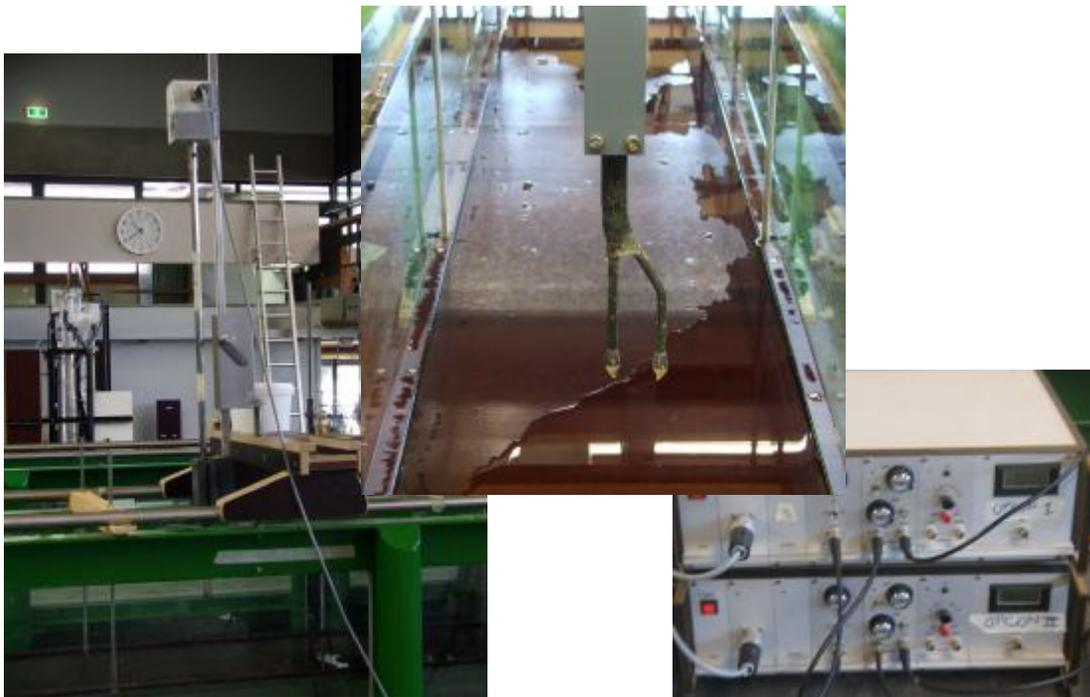
Figure F.7: OPCON concentration meter: probe, detail of probe and control units
