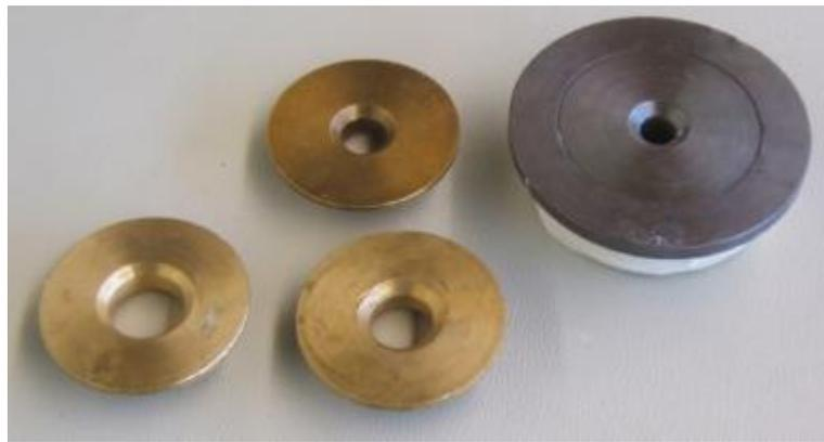
Figure G.6: Different flanges used in experiment, the dark one is already placed in the basis that was reused for every flange.
