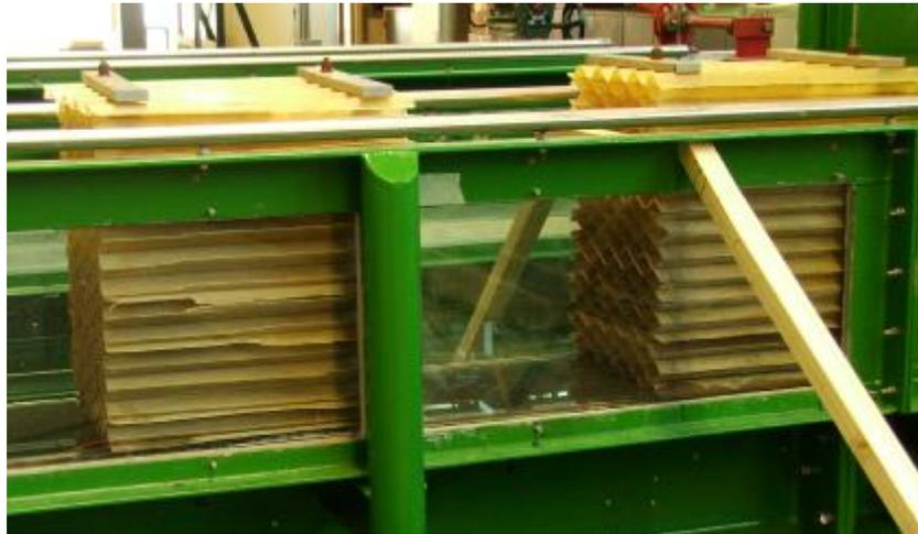
Figure H.2: Packs of corrugated sheets placed into the flume to prevent meandering.
