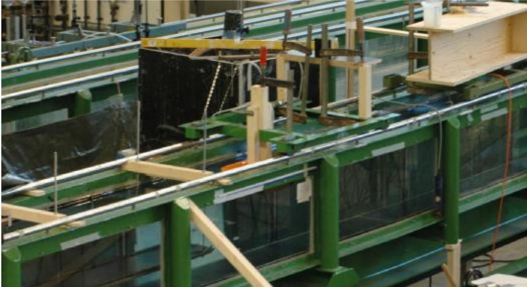
Figure G.2: Placing of the siphon in the experimental setup
