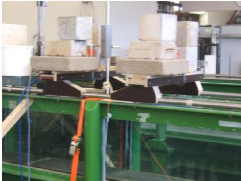
Figure H.6: Setup for Vectrino apparatus loaded with concrete blocks and lead bars
