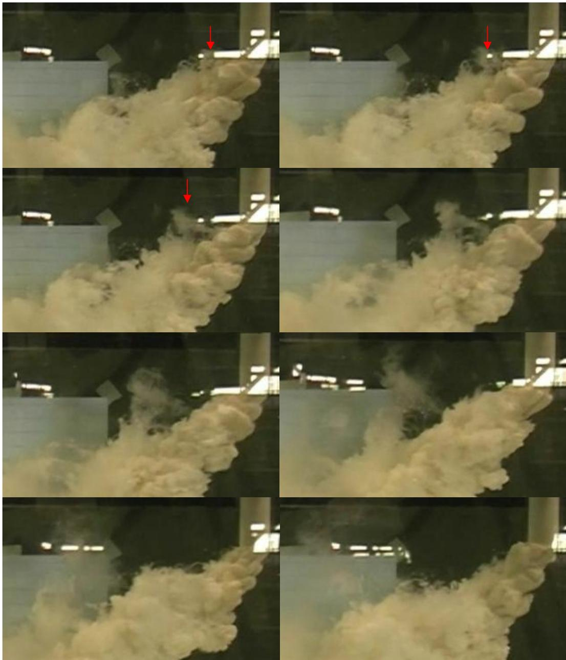
Figure 7.2: Series of subsequent pictures showing a vortex breaking from a plume
