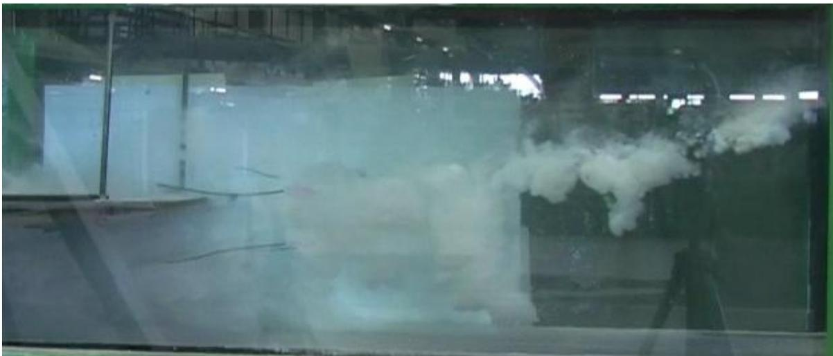
Figure 7.7: Plumes with varying overflow parameters behaving as separate clouds and puffs.
