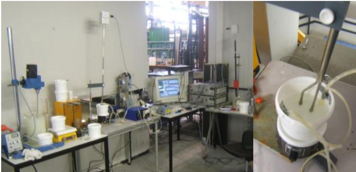
Figure F.8: Calibration setup to calibrate concentration meters, right: detail of the measuring bin
