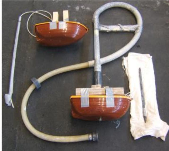
Figure G.8: Smaller siphons created for the experiments.
