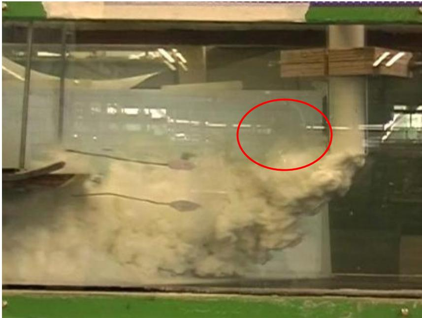
Figure 7.8: Recirculation of material in wake of pipe
