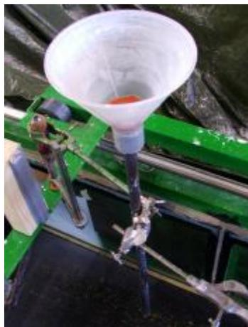
Figure 7.6: Overflow pipe with funnel constructed for variable overflow creation
