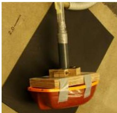
Figure E.4: Picture of the model ship used to prevent wake forming behind the pipe
