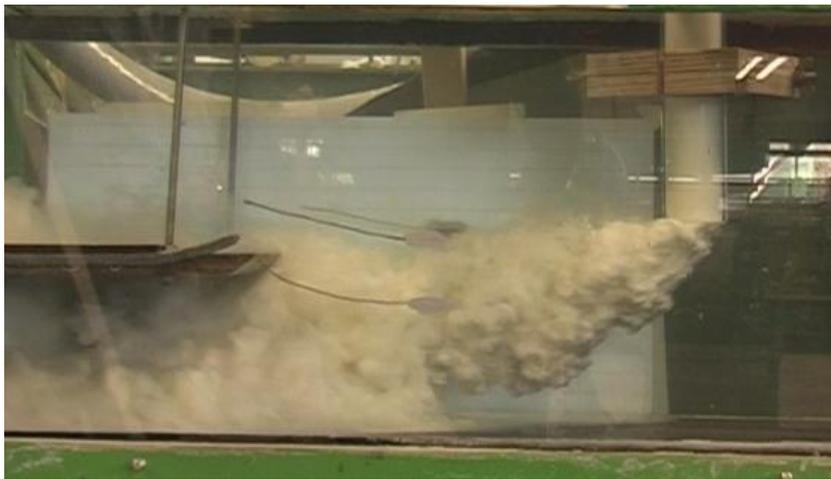
Figure J.1: Base case plume in experimental flume.
