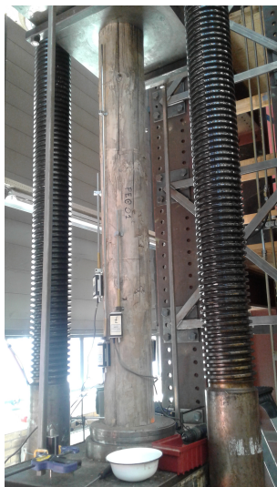
Figure B.5: Overview of the testpiece PEO01 before testing.
