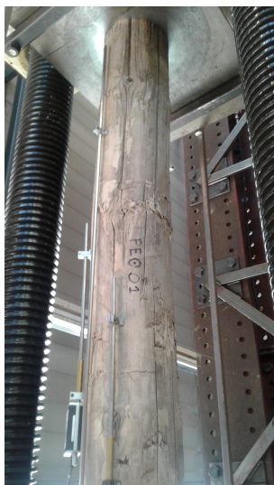
Figure B.6: Close-ups of the failing testpiece PEO01.
