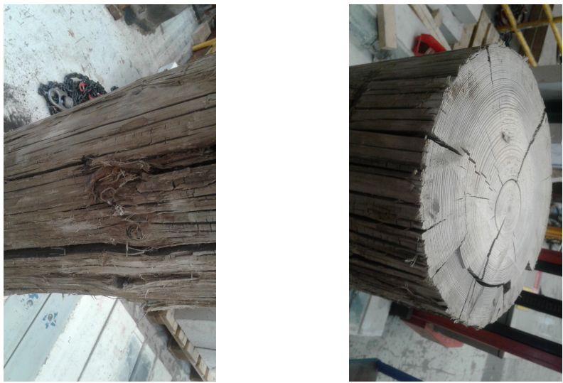
Figure B.44: Close-ups of the failing testpiece PKO0120 (left), after testing (right).
