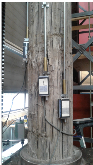
Figure B.52: Close-ups of the failing testpiece POA0140.
