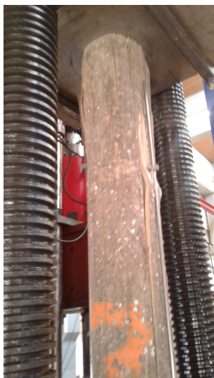
Figure B.32: Close-ups of the failing testpiece PJC0120.
