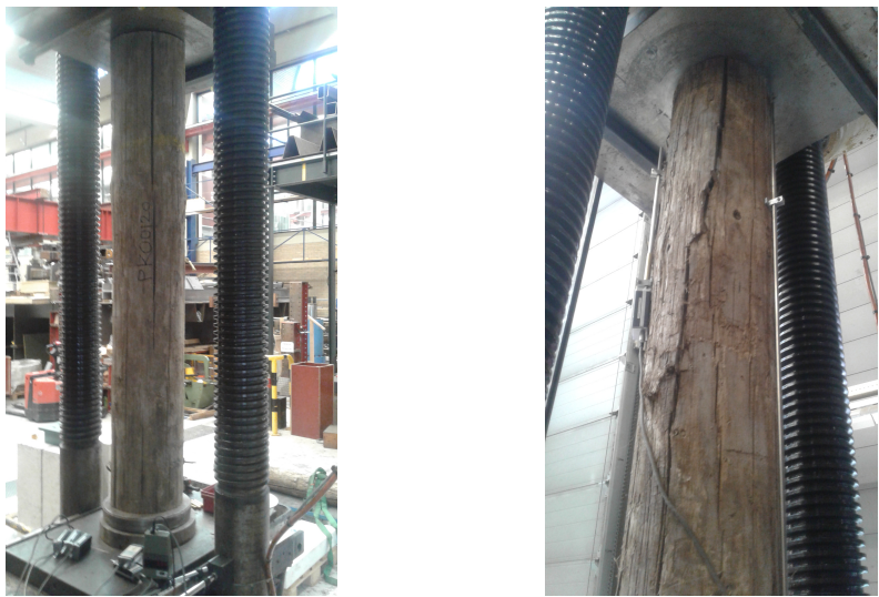
Figure B.43: Overview of the testpiece PKO0120 before testing (left), and during plasticity (right).
