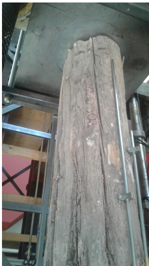
Figure B.59: Close-ups of the failing testpiece POC0120. Note the eroded top.
