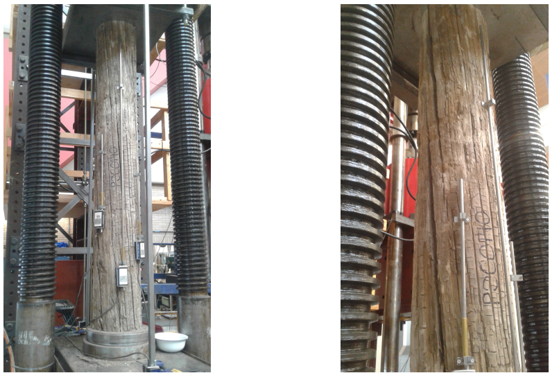
Figure B.62: Overview of the testpiece POC0140 before testing (left), and during plasticity (right).
