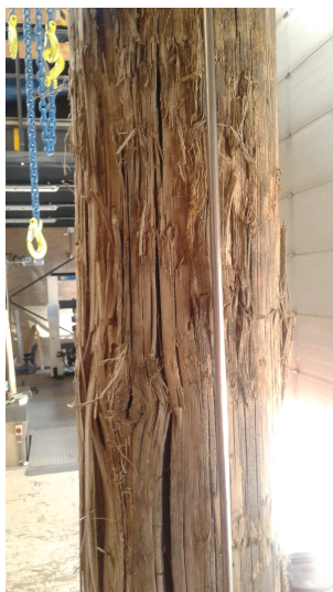
Figure B.55: Close-ups of the failing testpiece POA0750.
