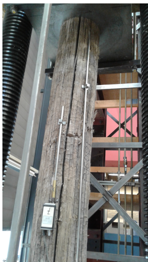
Figure B.36: Close-ups of the failing testpiece PJC0121.
