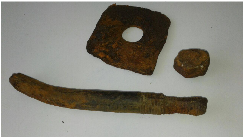
Figure 5.10: Overview of 3 different steel parts. Note the poor state of the threaded end of the bolt.
