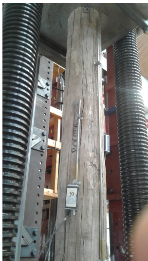
Figure B.80: Overview of the testpiece POC0742 before testing.
