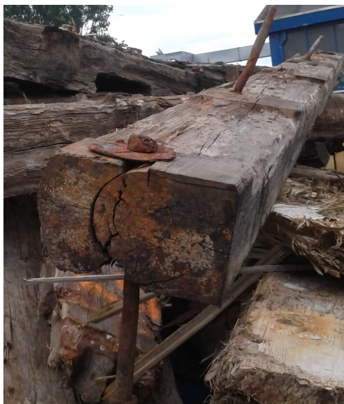
Figure 5.6: A hardwood capping beam. Note the difference in thickness along the profile and the cracks on the end grain. All hardwood capping beams are from wall section 3-1 and are constant in cross-section, the pins in the picture are from the connections to the piles.
