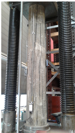
Figure B.21: Overview of the testpiece PGC0122 during plasticity
