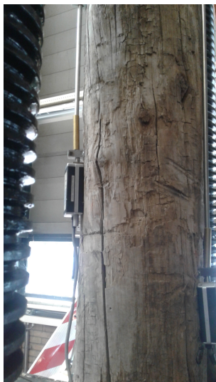
Figure B.63: Close-ups of the failing testpiece POC0140.
