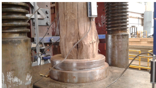
Figure B.81: Close-ups of the failing testpiece POC0742.
