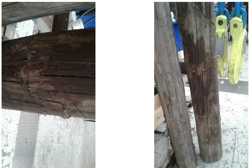
Figure B.73: Close-ups of the failing testpiece POC0721.
