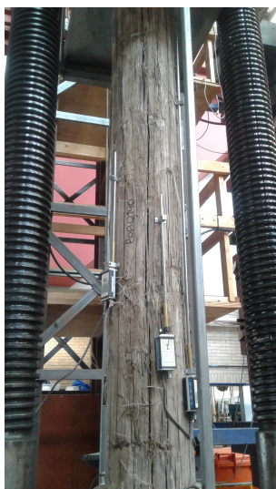
Figure B.51: Overview of the testpiece POA0140 before testing.
