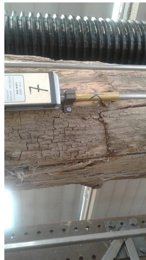
Figure B.59: Close-ups of the failing testpiece POC0120. Note the eroded top.
