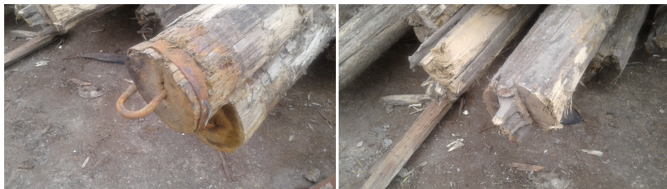
Figure 5.5: Pileheads; pin (left), mortise-and-tenon (right)
