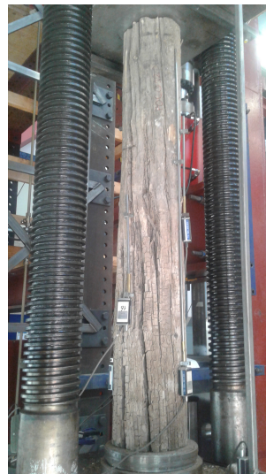
Figure B.58: Overview of the testpiece POC0120 before testing (left), and during plasticity (right).
