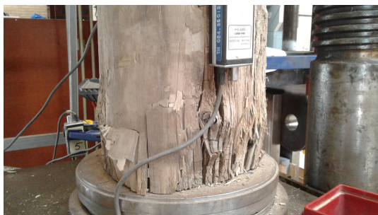
Figure B.22: Close-ups of the failing testpiece PGC0122.
