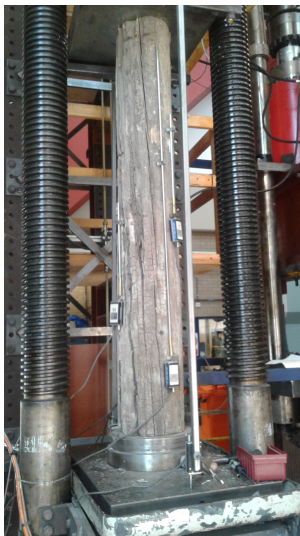
Figure B.58: Overview of the testpiece POC0120 before testing (left), and during plasticity (right).
