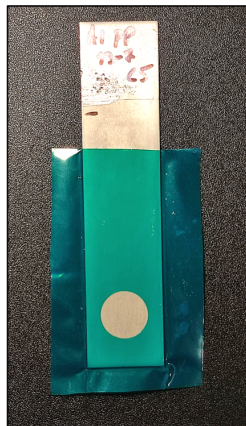
Figure 3.2: An example of a specimen used for the OCP and PP measurements.
