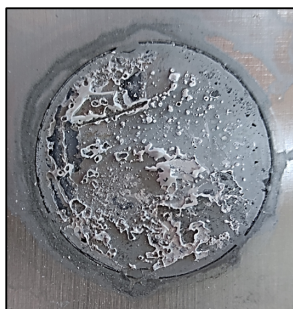
Figure 3.15: A pure zinc sample after potentiodynamic polarization when placed horizontally.
