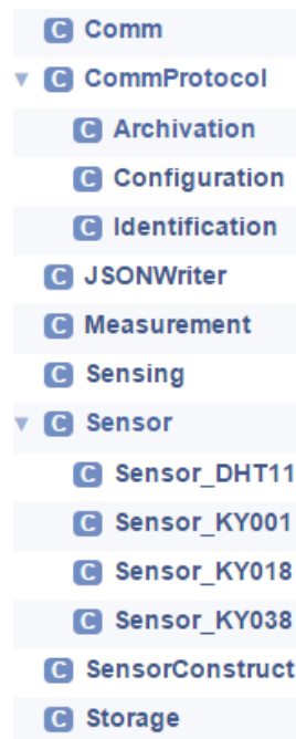
Figure 4.4: Class Hierarchy of the Arduino implementation (generated using Doxygen)
