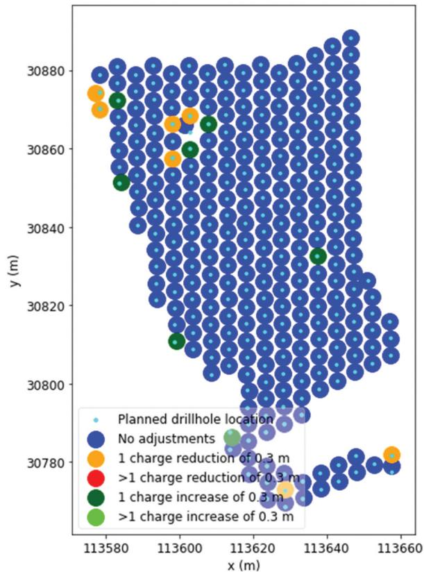
Figure 12. Charge adjustment solution for Nevada 2 dataset.
