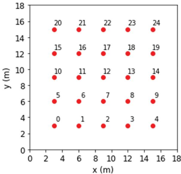
Figure 6. The 5 by 5 test pattern planned drillhole locations.
