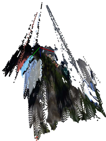
Figure 13: A point cloud extracted from a disparity image when an invalid camera calibration is applied.
