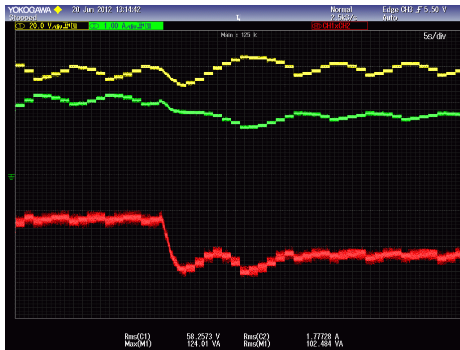
Figure 8.6: Shading test adaptive P&O, Voltage (yellow), Current (green), Power (red), 5 s/div
