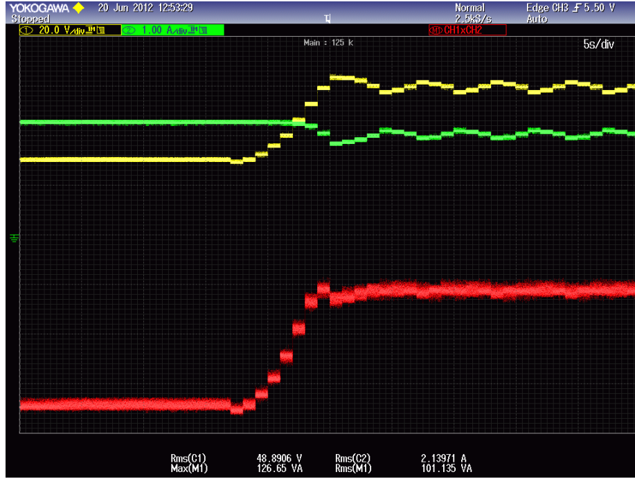
Figure 8.5: 70% test adaptive P&O, Voltage (yellow), Current (green), Power (red), 5 s/div
