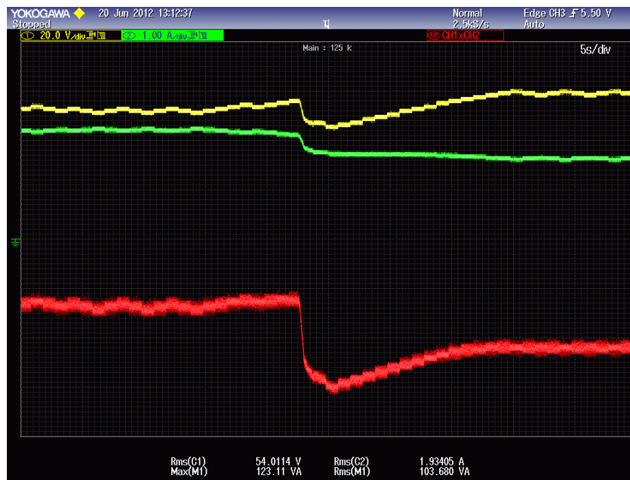
Figure 8.4: Shading test P&O, Voltage (yellow), Current (green), Power (red), 5 s/div
