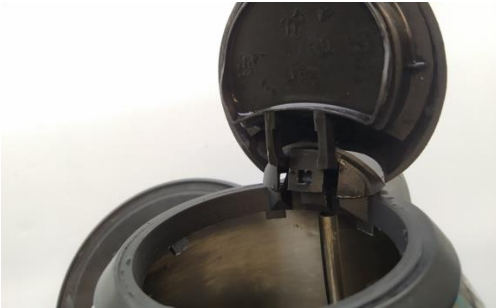
Figure 34 - Testing the fit and function of the top ring and switch inside the kettle.
