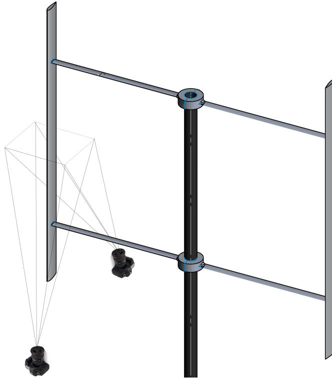
Figure 3.11: Multiple camera positions are used to remove the lower strut in the stitched velocity field.
