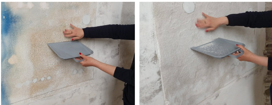
Fig. 9. Left: Panel A1: No loss of cohesion of the plaster; Right: Panel A2 significant sanding of the plaster; Situation 48 months (t48) after the application.
