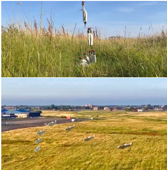
Figure 4.1: (Top) TRE-tailsitter executing a pivot takeoff, where it pitches up steadily off the ground by pivoting around its tail by thrust vectoring. (Bottom) Transition from hover to forward flight, captured at 0.1-second intervals.
