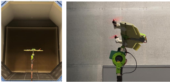
Figure 5.2: Wind tunnel experimental setup pictures showing the tilt-rotor tailsitter mounted on a six-axis force/torque sensor in the OJF wind tunnel[14], with a servo-driven mechanism to adjust angle of attack.
