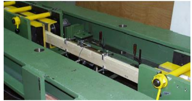
Figure 3: Testing device according to DIN EN 408 [11].
