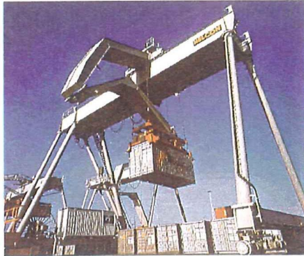
Rail mounted gantries (automated)
