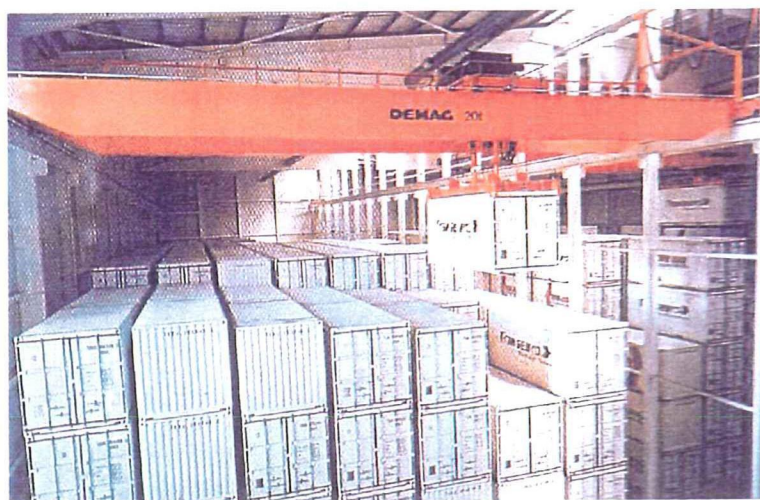
Figure 5: Underground storage of reefers
