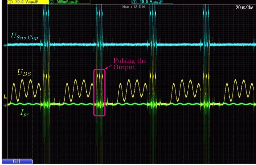
**Fig 5.35.** Output waveforms in case voltage at **Sns Fb** pin reduced to 1V.  $U_{dc} = 30V$ , aluminum pan and SPW47N60CFD.
