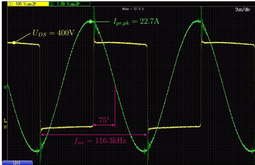
**Fig 5.31.** Achieved results in case of  $U_{dc} = 407V$ ,  $I_{dc} = 4.1A$ , aluminum pan and SPW47N60CFD.
