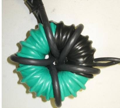
**Fig 5.8.** The matching transformer.
