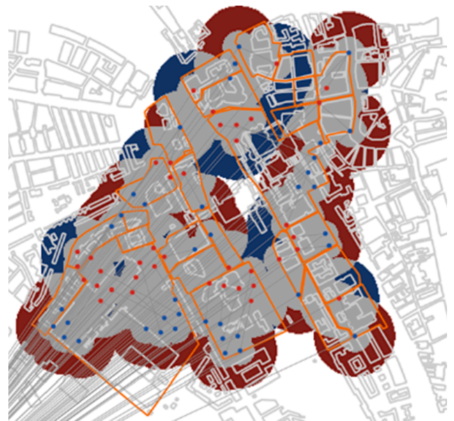
Fig. 9. Example output of the Agent Based model: placement of 39 well pairs (78 total wells).
