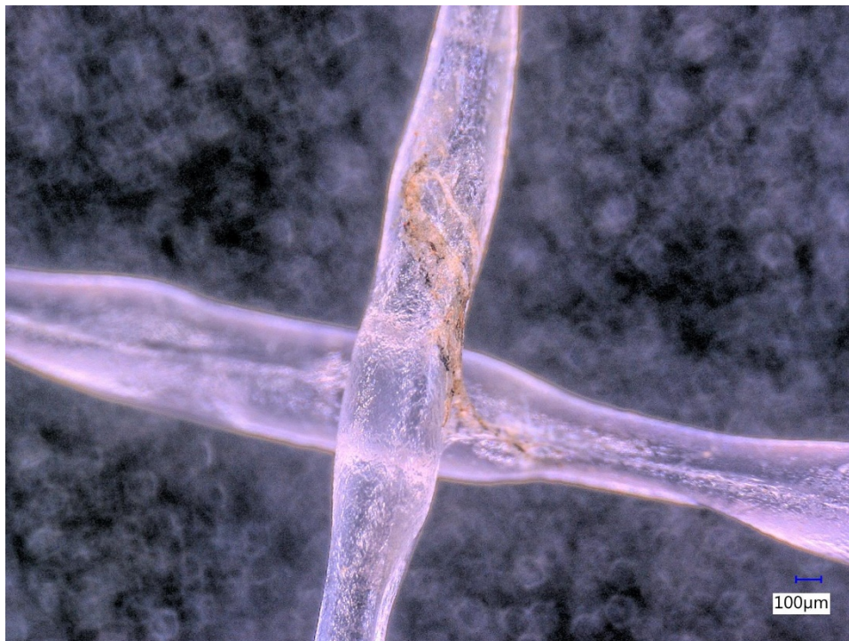
Figure 67: visual details of feed spacer after operation
