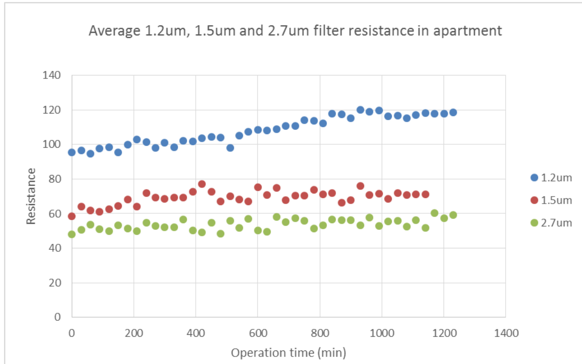
Figure 35: Average 1.2um, 1.5um, and 2.7um filter resistance operated in apartment condition
