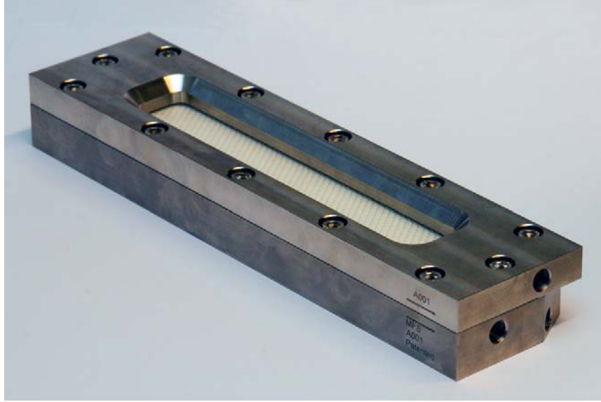
Figure 4: Side view of MFS (Vrouwenvelder, J., et al., The Membrane Fouling Simulator: A practical tool for fouling prediction and control. Journal of Membrane Science , 2006. 281(1-2): p. 316-324.)
