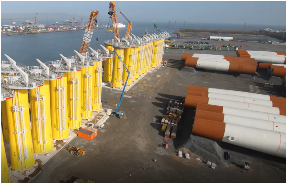
Figure 2.6: Monopiles (left) and Transition Pieces (right)
