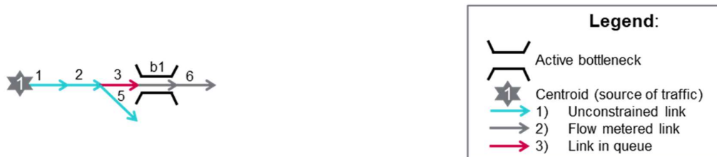
Figure 4: example where estimating demand matrices using method 1 and a single count on link 2 does not imply a positive effect on the fit on link 3
