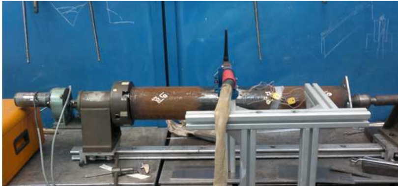
Figure 25 Figure shows test set up used for fusion welding in the vicinity of notch region using Metal Inert Gas welding machine (MIG).
