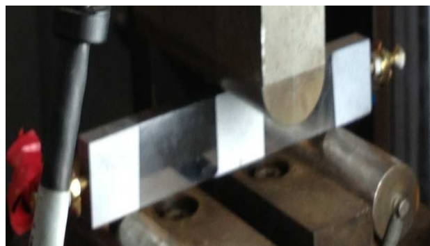
Figure 46 Three point bend fatigue test on notched strip specimen
