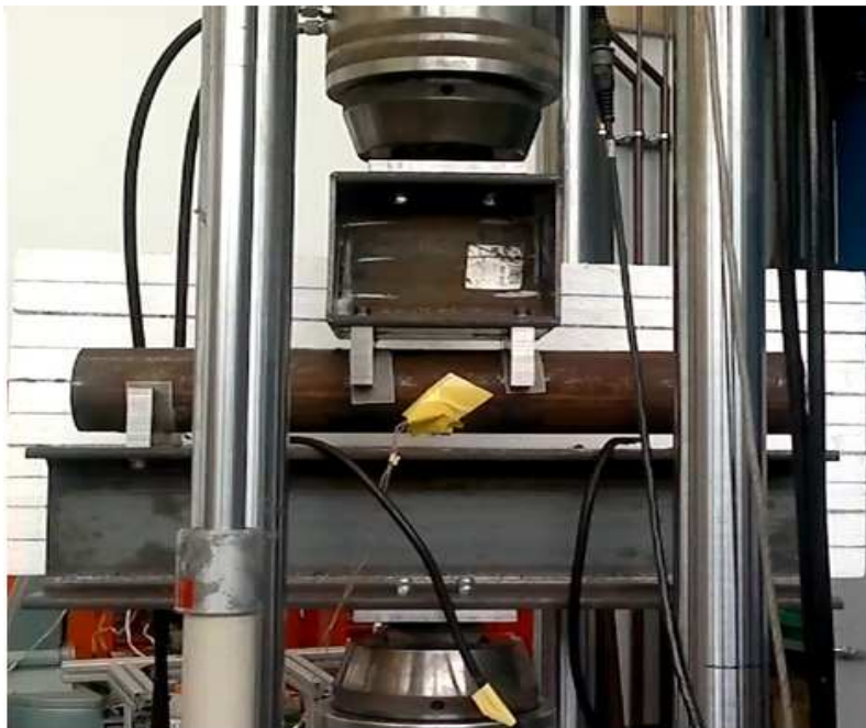
Figure 14 Pipe specimen with surface notch loaded in four point bend test-rig.
