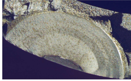
Figure 20 Figure shows the initial semi-elliptical notch and beachmarks produced during variable amplitude fatigue test in cracked region in pipe specimen.
