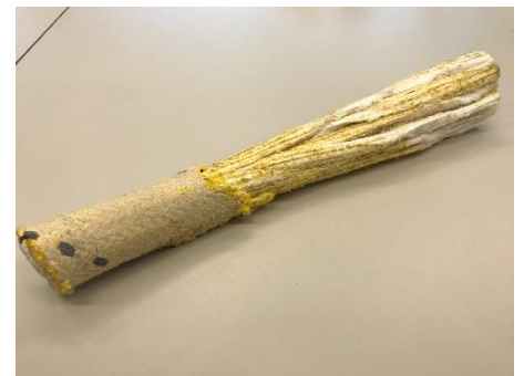
Figure 15: A unsuitable rope for growing seaweed on due to the rope shield. Source: self-made image.
