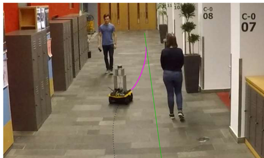
Fig. 1. The faculty corridor was the scenario used to evaluate the capabilities of our method to avoid dynamic obstacles.
