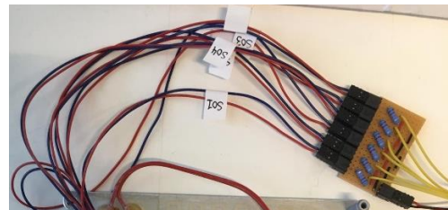
Figure 43. Schematic and Actual Temperature sensor configuration. The 5V (max 500 mA) signal from the Arduino board first crosses the NTC (variable resistor) and then either goes back to the Arduino (AnalogRead to read output voltage) or continues via a constant resistor (12k \Omega ) to the ground.
