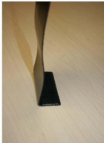
Fig 10: sample of IXIS strip shaped to the contour of 5th door of Superbus
