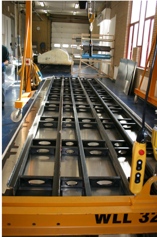
Fig 8: assembly of the lower plate and longitudinal and transversal beams
