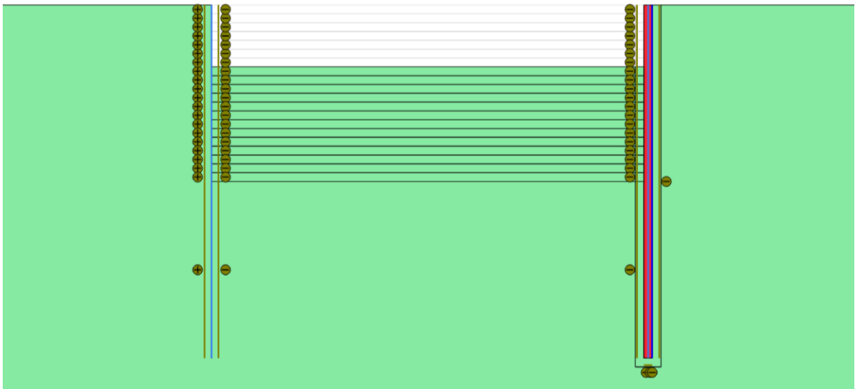
Figure 50: Model set-up excavation with for demonstration; left a Plate element and right a reinforced volume element.
