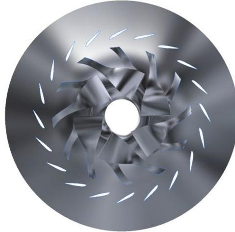
Figure 5.5: MTT Impeller with 20 Vanes Airfoil Shaped Low-Solidity Vaned Diffuser
