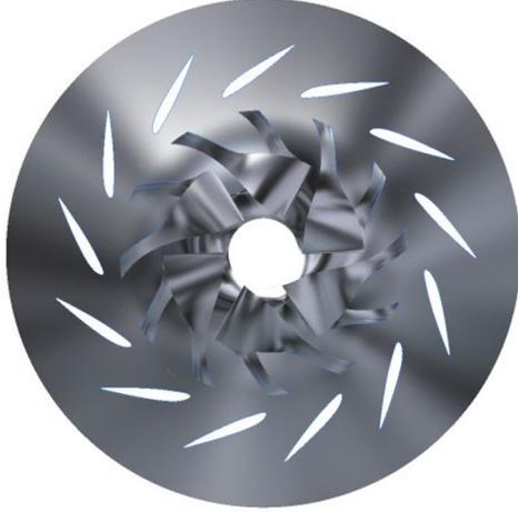
Figure 5.4: MTT Impeller with 13 Vanes Airfoil Shaped Vaned Diffuser
