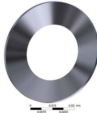
Figure 4.2: MTT Vaneless Diffuser
