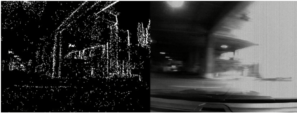
Figure 2.4: Fast moving scene captured with an event-based camera (left side) and with a grayscale frame-based camera (right side). Retrieved from Chen (2017).
