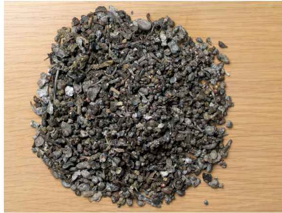
Figure 1.7: An examples of a product from BA, the 2-6 mm heavy non-ferrous metals.
