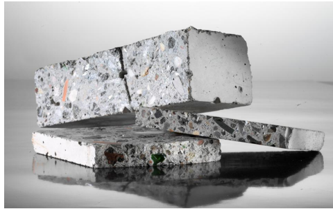
Figure 6.5: Concrete sample made with 30% of AEB aggregate mixture.
