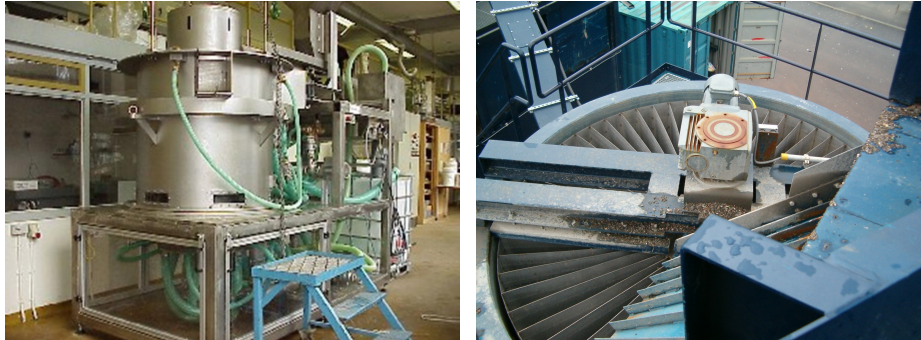
(a) Kinetic gravity separator (KGS) as used in the Pilot plant I. (b) View of the gravity separator from the top-the material input, Pilot II.
