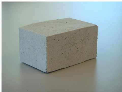
Figure 6.6: Lime-sand stone made from AEB sand product (in 2004).
