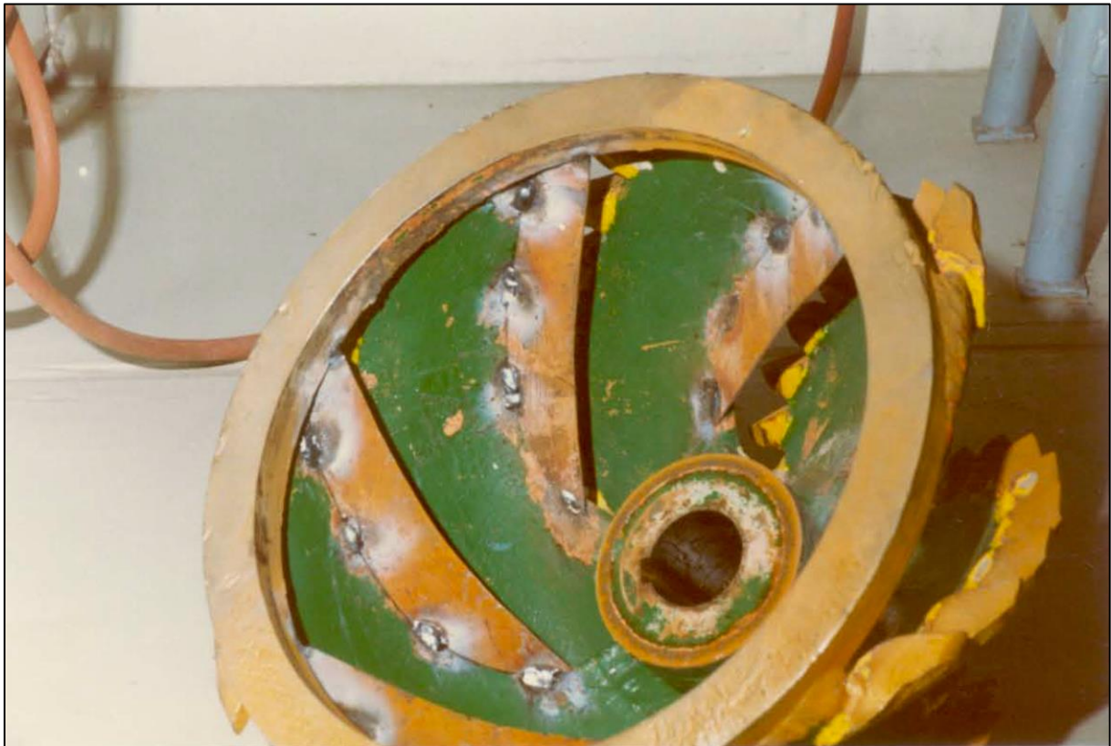
Figure 7-47: Skirts mounted inside the crown cutter head.
