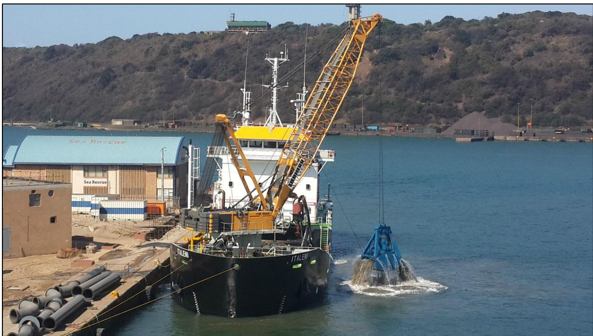
Figure 12-1: Self-propelled grab hopper dredge.
