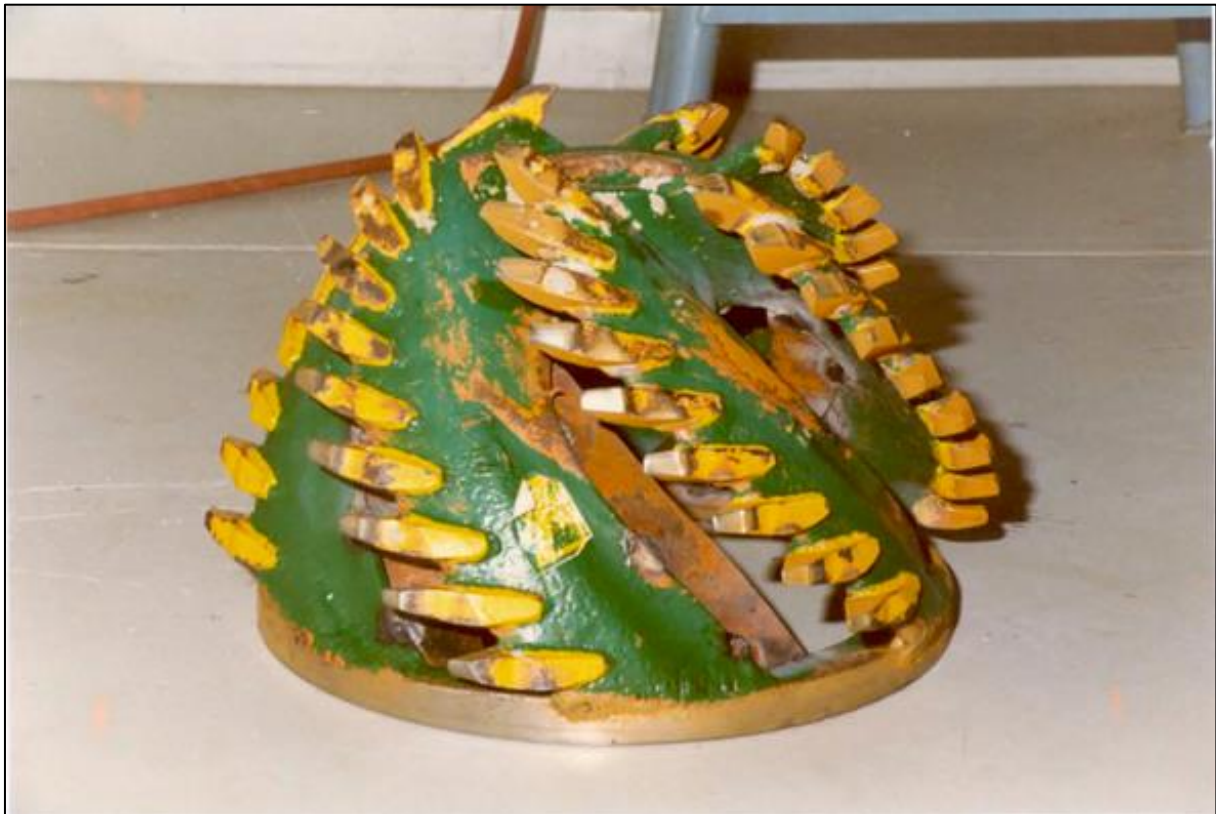
Figure 7-45: The crown cutter head used by Miltenburg (1982).
