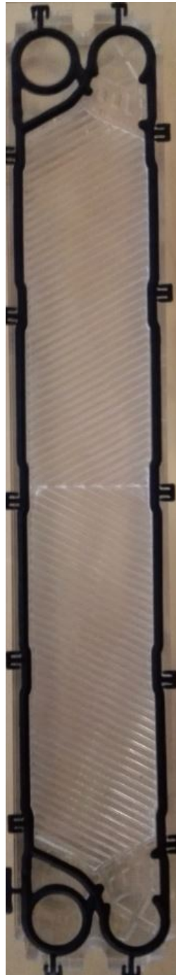
(a) The fabricated transparent corrugated plate, with gasket.
