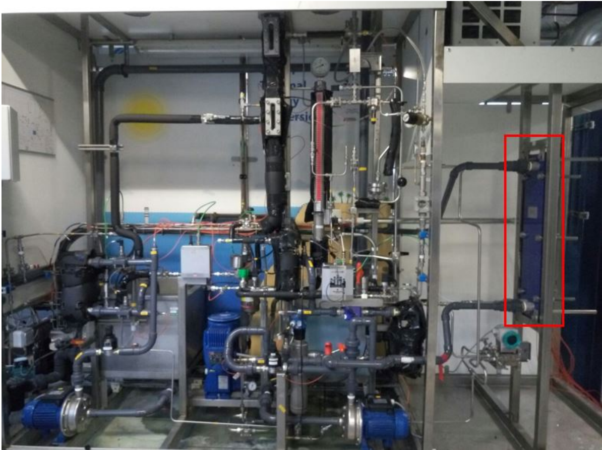
Figure 3.10: Image of the OTEC-demo, with the constructed extension. The red rectangle shows the location of the new condenser.
