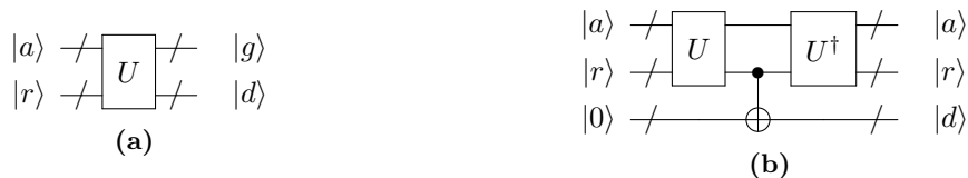
Figure 1.6: Method to avoid garbage production in a circuit. The registers |a\rangle , |r\rangle , |g\rangle and |d\rangle are respectively the ancillae, the register, garbage output and desired output. The operation U^\dagger is defined as the inverse of operation U .
