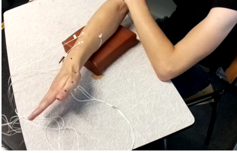
Fig. 3: The wired sEMG electrodes attached to the right arm of a participant. Black dots on the thumb indicate marker locations used for labeling in the DeepLabCut software.
