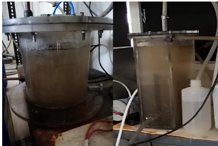
Figure 17 CSTR and Filtration Unit Before Aeration
