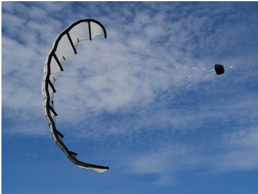
Figure 2.4: LEI DelftV3 kite with bridle system, KCU and tether LEI DelftV3 kite with bridle system, KCU and tether (Photo: R. Schmehl)
