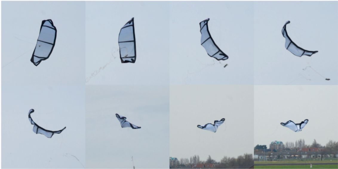
Figure 3.4: Rupture of the weak link leading to entanglement and stable but non-steerable descend
