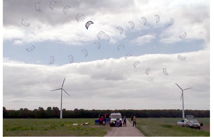
Figure 2.2: Kite flying figure-of-eight maneuver in the power zone during traction phase [11]
