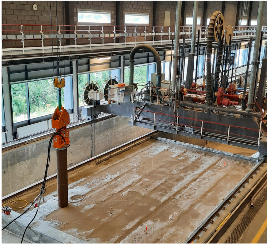
Fig. 1. The first pile placed on the soil surface prior to installation in the large soil tank of Deltares.
