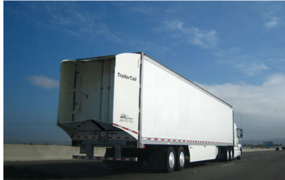
Figure 1.6: Example of base flaps applied on a heavy-duty vehicle [20].
