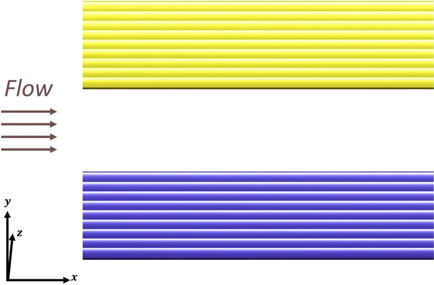
Figure 2.10: Different angle of view of the sinusoidal roughness with the direction of travel being in the spanwise direction, normal to the flow.
