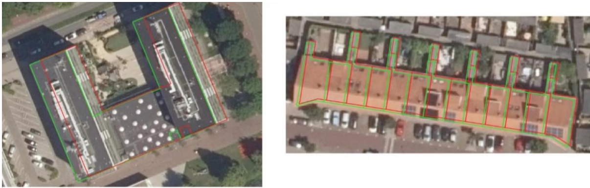
Figure 18. Misalignment between BAG footprint and Aerial Image. A property that compounds a building by itself (left), a group of properties that compound a single building (right).
