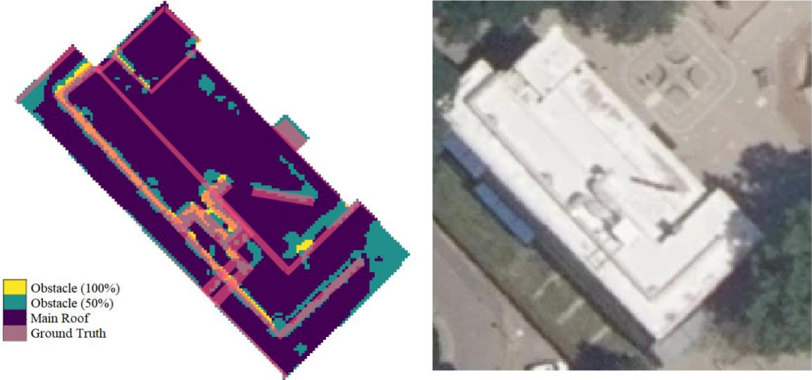
Figure 36. Comparison between the obstacle detection method with automatic alignment and the ground truth with the image of the respective building.
