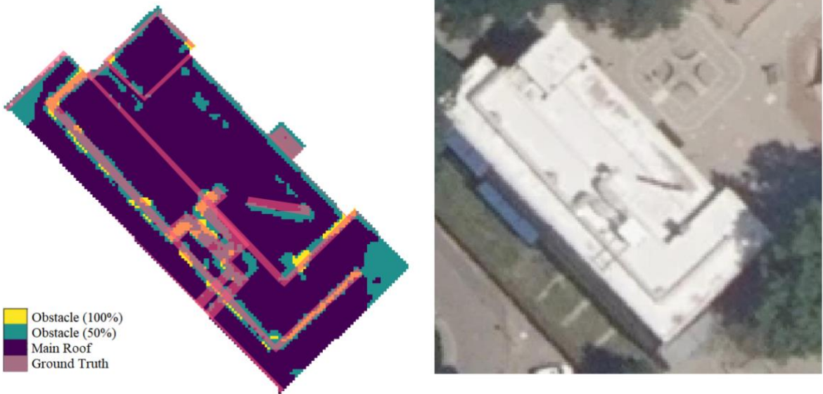
Figure 35. Comparison between the obstacle detection method with manual alignment and the ground truth with the image of the respective building.
