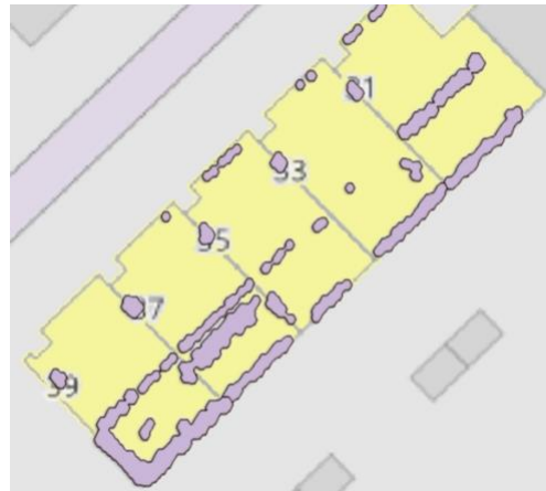
Figure 12. GeoJSON output, storing the obstacle polygons' geometry, the buildings' identificatie and their CityObject id from the CityJSON format.
