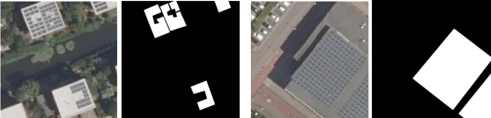
Figure 25. Examples of training image pairs for solar panel detection model.
