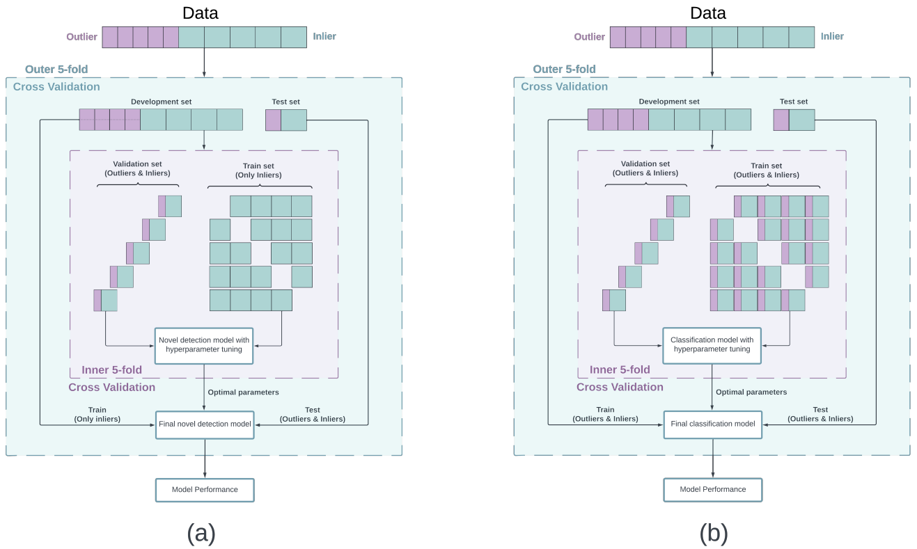
Figure 2.3: Visual representation of the 5-fold nested cross-validation strategy for (a) novelty detection and (b) classification. For novelty detection, the algorithm trains on only the inliers (purple), and for classification, both the inliers and outliers are used for training. Although not explicitly represented for clarity, each fold contains data of a unique subject.
