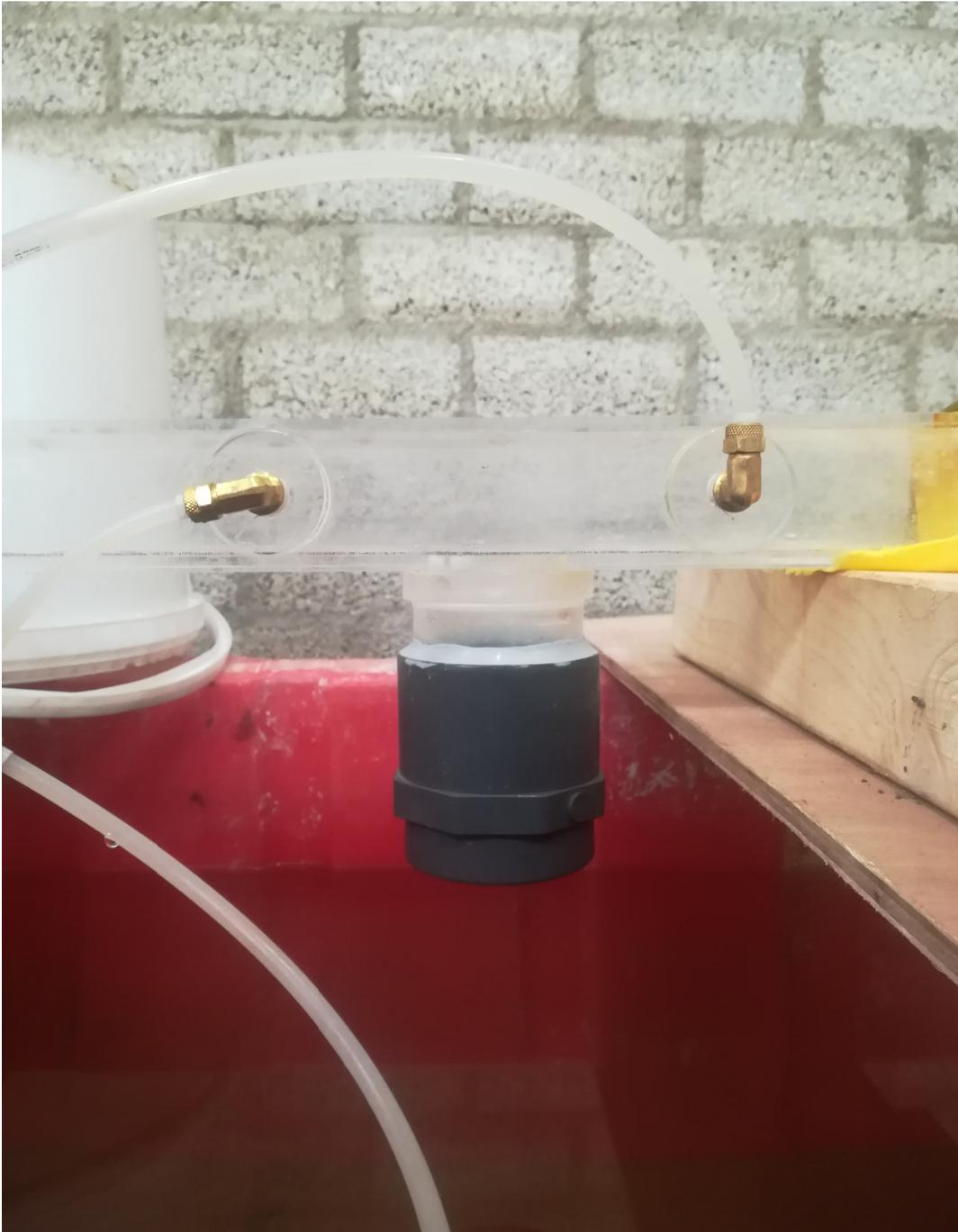
Figure H.8: Result soil feeding mechanism and polyflow connectors
