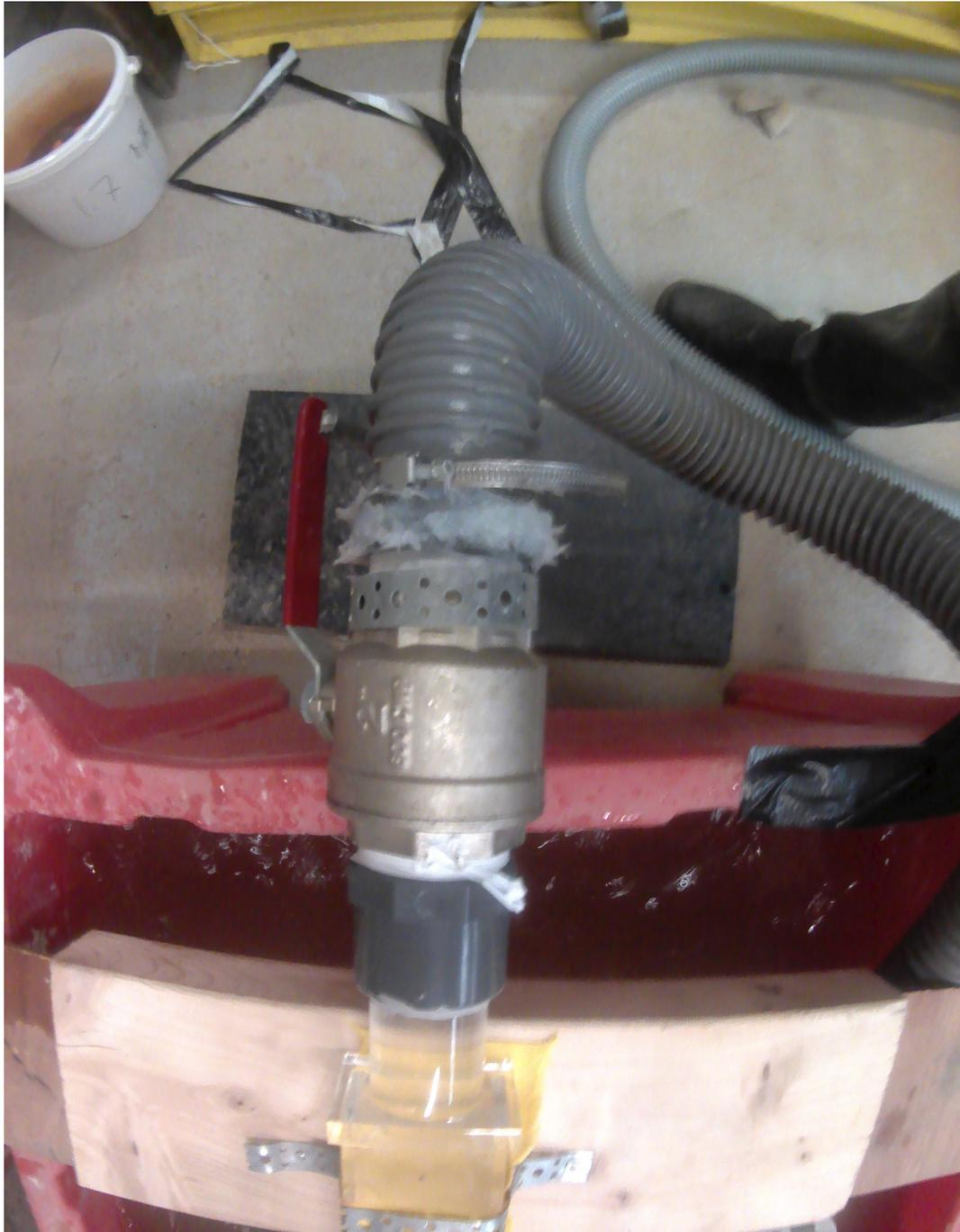
Figure H.5: Result connection round to rectangular tube
