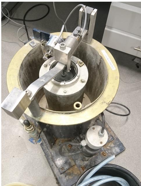
Figure 2.24: Photo of Erosion centrifuge at Deltares (Alkemade and Kruk (2018))
