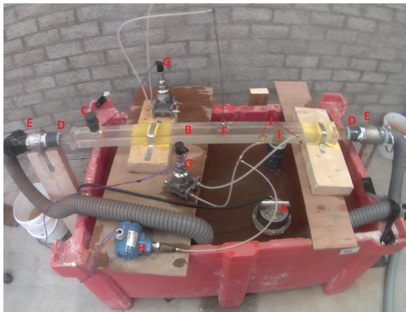
Figure 3.1: End result Erosion Function Apparatus
