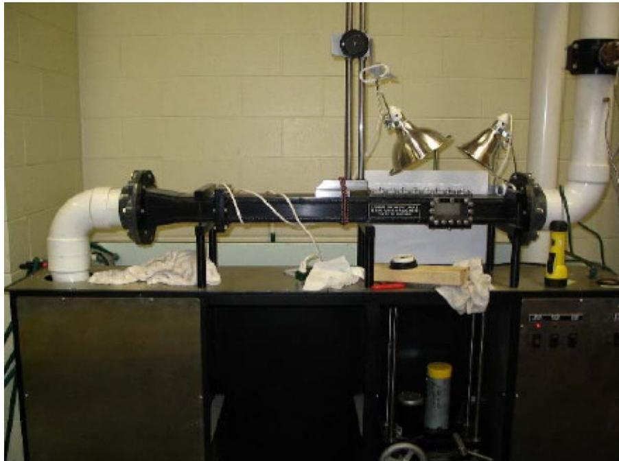
Figure 2.27: photo of Erosion function apparatus (M.E. Walker III (2013))
