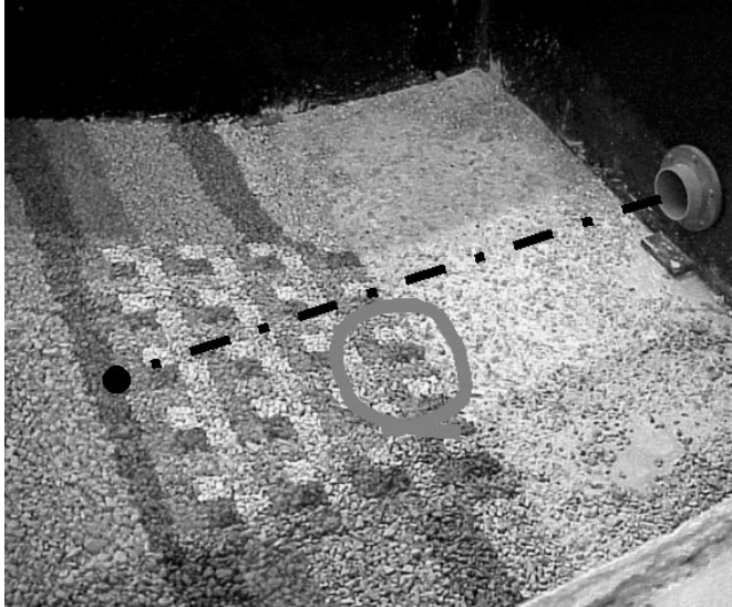
figure 7, damage location on the slope (circle) in the ducted propeller model and the intersection of the jet-axis with the slope (black dot).
